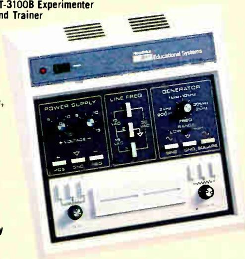
Solderless bread-board sockets for circuit building
