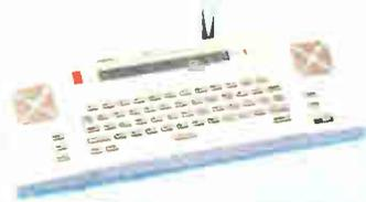
A hand-held wireless remote control console with full ASCII keyboard for manually controlling and remotely programming HERO 2000 from up to 100 feet away
