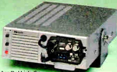
Slip handheld into the Console for mobile operations
