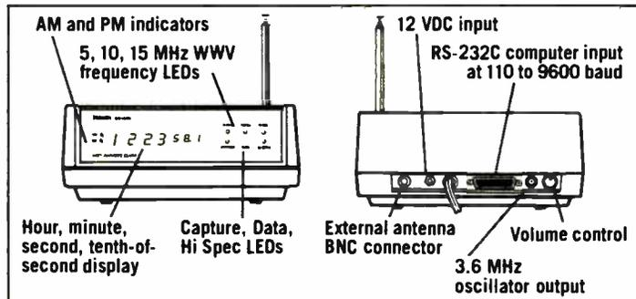
An RF receiver scans the 5, 10 and 15 MHz frequencies of WWV and locks onto the strongest signal. A selectable audio monitor permits you to listen to the audio broadcast on these frequencies. To improve reception of WWV frequencies, an external antenna is recommended but may not be required in your area.
