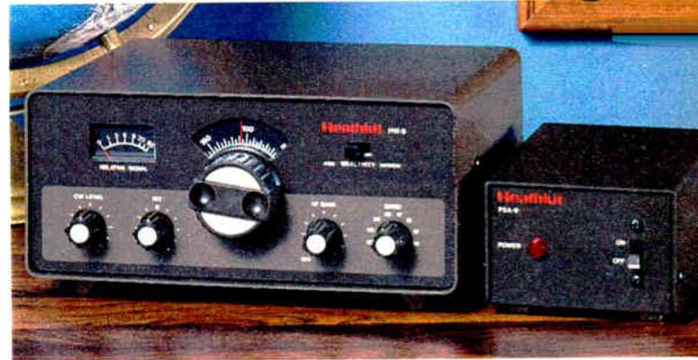
**RECEIVER: Sensitivity:** 0.2  $\mu$ V for readable signal; 0.5  $\mu$ V or less for 10 dB S + N/N. **Selectivity:** Wide, 1 kHz max. @ 6 dB; Narrow, 250 Hz @ 6 dB. **Dynamic Range:** 85 dB. **Image & IF Rejection:** 60 dB, min. **Audio Hum Noise:** - 60 dB. **Audio Output:** 1 watt into 8 $\Omega$ .
