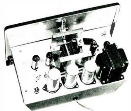
*A heavy-duty transformer, high filtering along with shielding both above and below the chassis assures purity of waveform output. All adjustments are conveniently made from top of chassis.*
