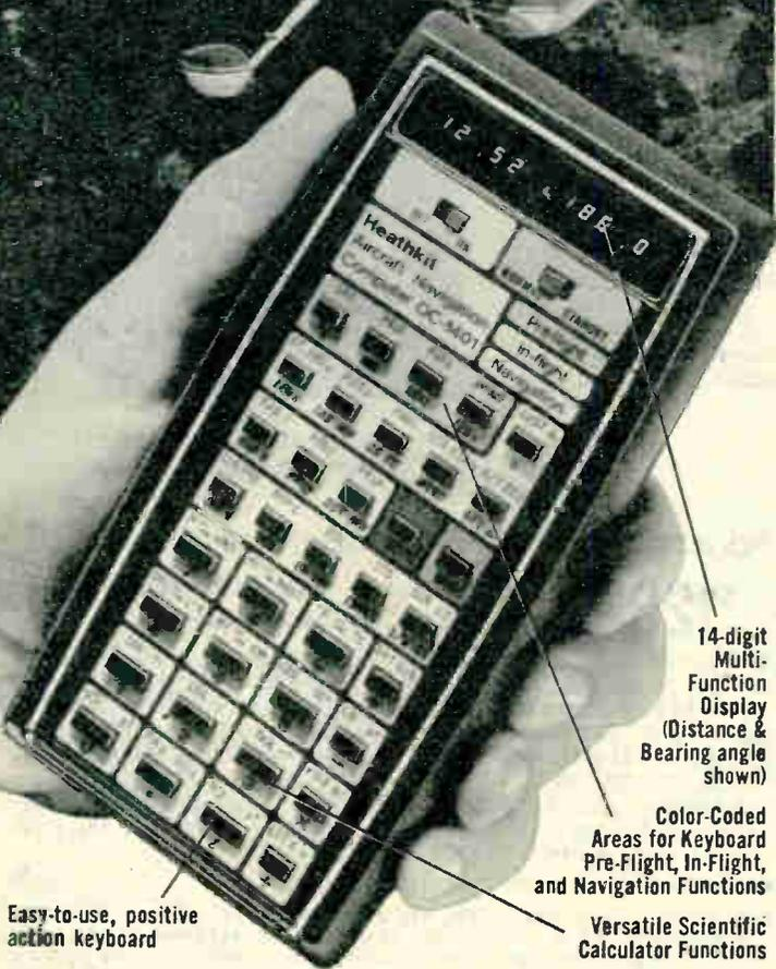
14-digit Multi-Function Display (Distance & Bearing angle shown)
