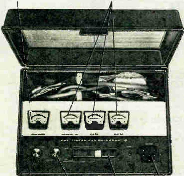
**Heater Adjust Control.** Sets voltage at CRT cathode for precise testing.
