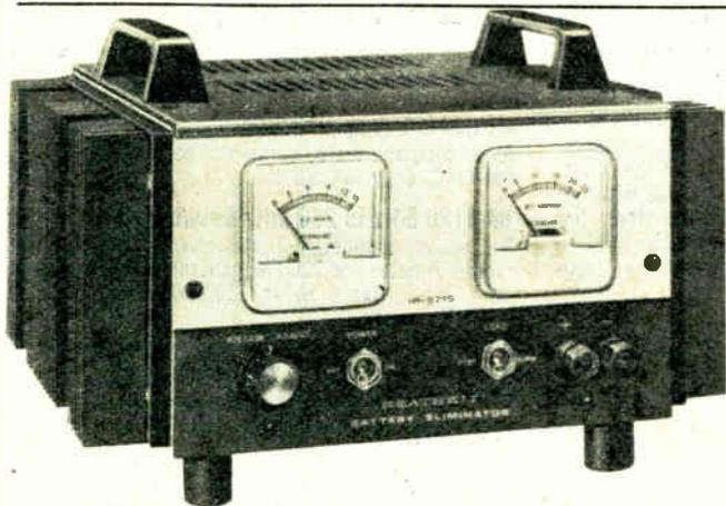
**IP-2715 SPECIFICATIONS:** Output Voltage: variable from 9-15 VDC. Output Current: 12 amps continuous, 20 amps intermittent (per derating curve in manual). Ripple: less than 1% at full load. Regulation: less than 2% variation from no load to full load. Fuses: 7A, 3 AG slow-blow primary; 20A, 3 AG output. Power Requirement: 110-130 VAC, 7A or 220-260 VAC, 3.5 A, 60/50 Hz. Dimensions: 5 3/4" H x 11" W x 11" D.
