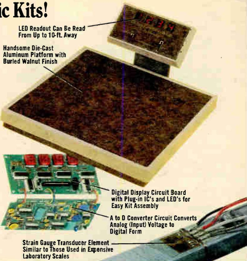
LED Readout Can Be Read From Up to 10-ft. Away
