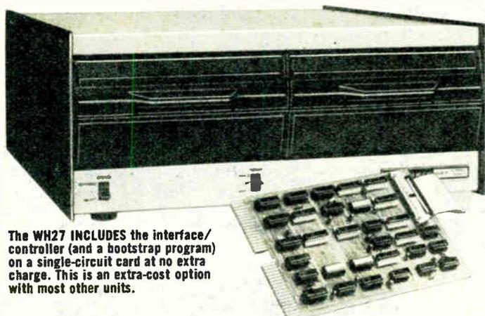
The WH27 INCLUDES the interface/controller (and a bootstrap program) on a single-circuit card at no extra charge. This is an extra-cost option with most other units.
