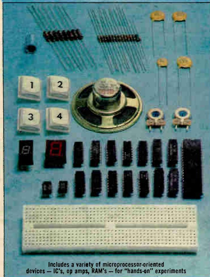
Includes a variety of microprocessor-oriented devices — IC's, op amps, RAM's — for "hands-on" experiments
