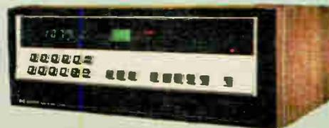
**AJ-1510A SPECIFICATIONS: Antenna:** 75 or 300 ohm. Sensitivity: Less than 1.8  $\mu$ V. Selectivity (alternate channel): Greater than 95 dB. Capture ratio: Less than 1.5 dB. Harmonic distortion: Less than 0.3%. IF rejection: Greater than 95 dB. Spurious rejection: Greater than 90 dB. Stereo channel separation: 1,000 Hz, 40 dB; 80 Hz, 25 dB; 10 kHz, 25 dB; 15 kHz, 20 dB. Audio output level: fixed: 1.2 V rms nominal (with 100% mod.). Power Requirement: 120/240 VAC, 60/50 Hz, 50 W.
