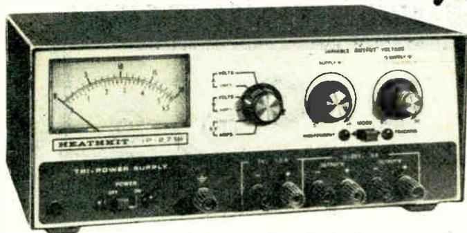
**IP-2718 SPECIFICATIONS:** Regulation: Load: less than 0.1% variation from no load to full load on 20-volt supplies; less than 2% variation from no load to full load on 5-volt supply. Line: less than 0.2% variation for line voltage change of 10 volts on 20 volt supplies; less than 0.15% variation for line voltage change of 10 volts on 5-volt supply. Power Requirement: 100-135 or 200-270 VAC, 60/50 Hz, 100 watts full load. Dimensions: 4 1/2" H x 10 3/4" W x 9" D.
