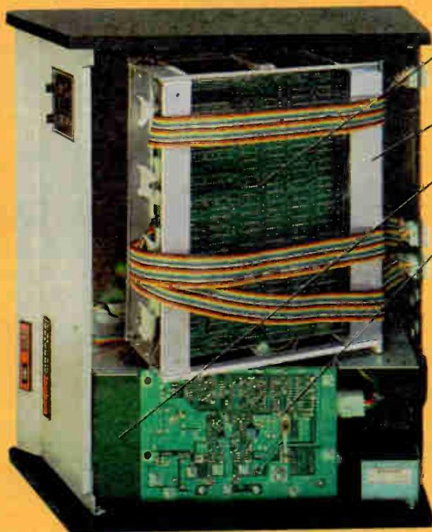
Card cage with backplane accommodates up to eleven accessory cards in addition to LSI-11/2. The card cage swings up for easy access and service even while the H11A is operating. Accessory boards slide directly into card guides with all connectors supplied.
