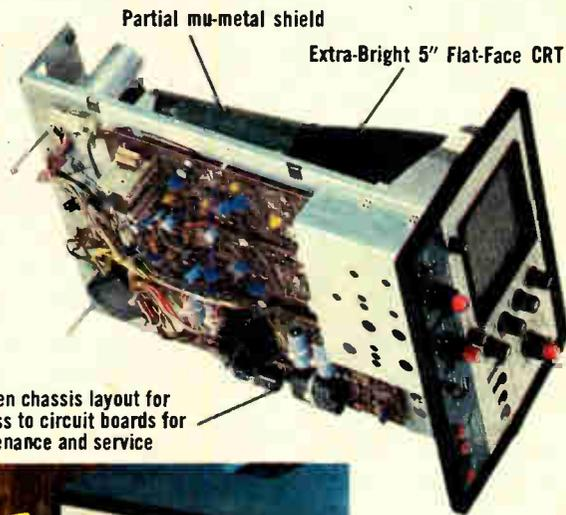
Wide-open chassis layout for easy access to circuit boards for maintenance and service
