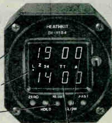
4-digit red LED displays with automatic dimming.
