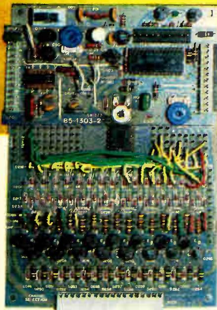
The "heart" of the GR-2000 is the channel selector circuit board. It provides the direct electronic tuning, the dot generator for color alignment, and positions and controls the channel display.
