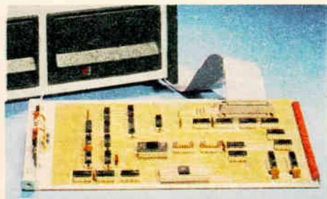
**The WH17 INCLUDES the Interface/Disk Controller Circuit Board — An Extra Cost Option with Most Other Units.**
