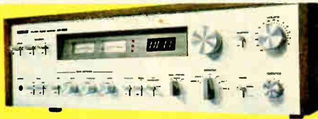
switch bypasses tone controls to provide the flattest possible frequency response. High and low, maximally flat response filters with 12 dB per octave roll-off minimize signal reduction in the passband and maximize attenuation of undesired signals beyond the 3 dB frequency. They are among the best response filters you can find at any price.
