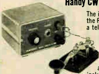
The ideal way to build up your code speed for the FCC exam, this practice oscillator features a telegraph key, phone jack, built-in speaker, plus volume and tone controls. Once you get your license, the HD-1416 can serve as a side tone oscillator for any transmitter using grid block keying. Dimensions: 2 $\frac{3}{8}$ " H x 4 $\frac{1}{8}$ " W x 4 $\frac{3}{8}$ " D. Operates on a single 9 V transistor battery (not included). Easy-to-build first-time kit.
