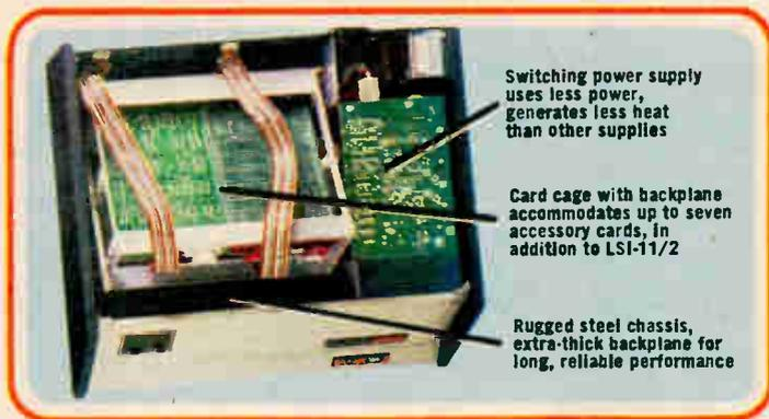
Switching power supply uses less power, generates less heat than other supplies
