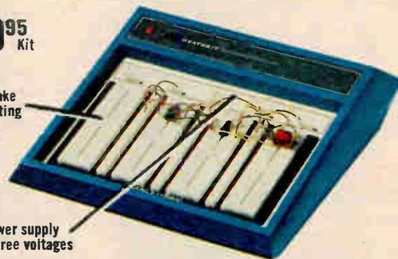
Built-in power supply provides three voltages
