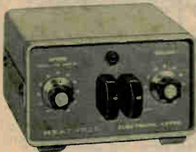
Your CW transmissions will be 100% copy with the HD-1410, because sending code is easy, whether you're operating base or portable. The dot and dash paddles travel and tension are easily adjustable. When the two paddles are treated as one, the HD-1410 operates like a single-paddle keyer with dot and dash memories. Iambic operation forms most characters with reduced wrist movement. Dots and dashes are self-completing and
