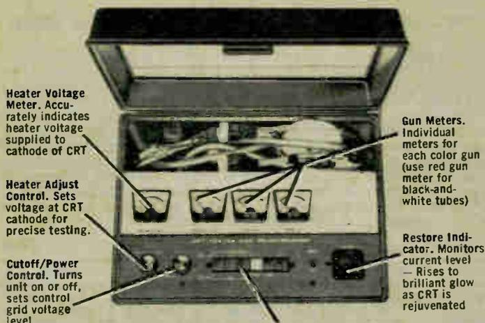
Heater Voltage Meter. Accurately indicates heater voltage supplied to cathode of CRT
