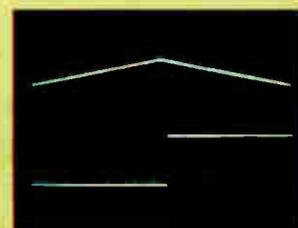
The delayed sweep takes the user selected portion of the waveform (intensified in the left picture) and magnifies it the desired number of times for closer examination (right picture).
