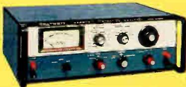
Outstanding sensitivity and bandwidth to let you measure Total Harmonic Distortion at levels as low as 0.03%, from 5 Hz to 100 kHz, with 5% full scale accuracy. Can also function as an AC voltmeter, with 1 mV to 300 V full scale capability. Not for use in strong
