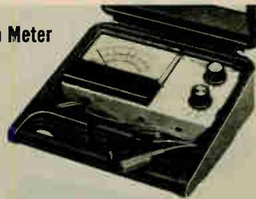
**CM-1073 SPECIFICATIONS:** Dwell meter: Three dwell scales: 8 cyl., 10-45 degrees; 4 cyl., 20-90 degrees; 6 cyl. & 3 cyl. x 2, 25-60 degrees. Tachometer: Two RPM ranges; Low range — 0-1500 RPM; High range — 0-2500 RPM. Dimensions: 4 $\frac{1}{4}$ " H x 8 $\frac{1}{2}$ " W x 7 $\frac{1}{4}$ " D.
