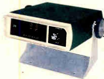
MI-101 SPECIFICATIONS: Accuracy:  $\pm 2\%$ ,  $\pm 1$  digit. Current drain: 300-500 mA. Power: 10-17 VDC @ 500 mA. Dimensions: 2 1/4" H x 6 1/2" W x 8 1/2" D (less gimbal).
