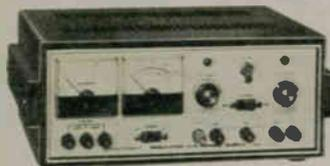
Provides 0-400 VDC at 0-100 mA continuous (125 intermittent) with excellent line and load regulation. Features front panel voltage and current meters, and built-in circuit protection. Binding posts are insulated from chassis. 120/240 VAC. 5¼" H x 13¾" W x 11" D.
