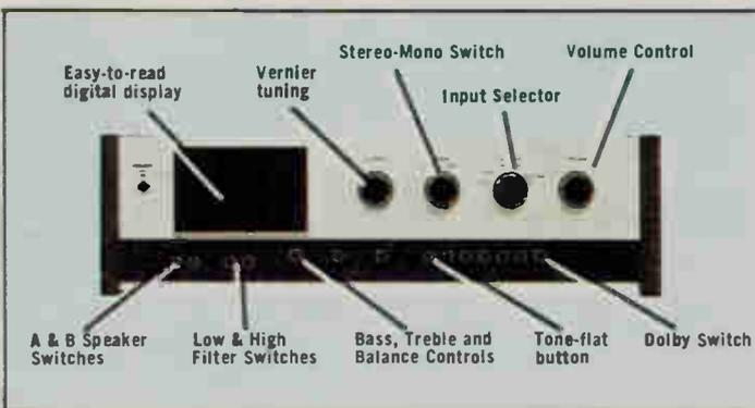
Add the AA-1515's low-distortion power needed to drive speakers to live performance volume levels. Same specs as the AR-1515 amplifier section below, except IM is less than .08%. Power Requirement: 120/240 VAC. Measures: 6 $\frac{1}{2}$ " H x 17 $\frac{1}{2}$ " W x 14 $\frac{1}{4}$ " D.
