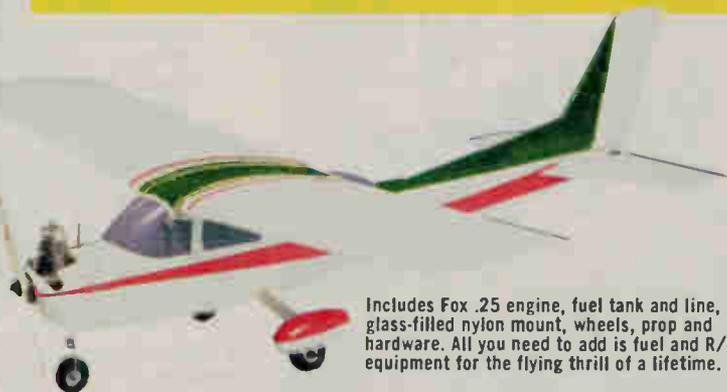
Includes Fox .25 engine, fuel tank and line, glass-filled nylon mount, wheels, prop and hardware. All you need to add is fuel and R/C equipment for the flying thrill of a lifetime.
