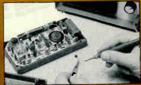
**INITIAL TESTING:** Before final assembly, you test the kit to insure that it is operating properly.
