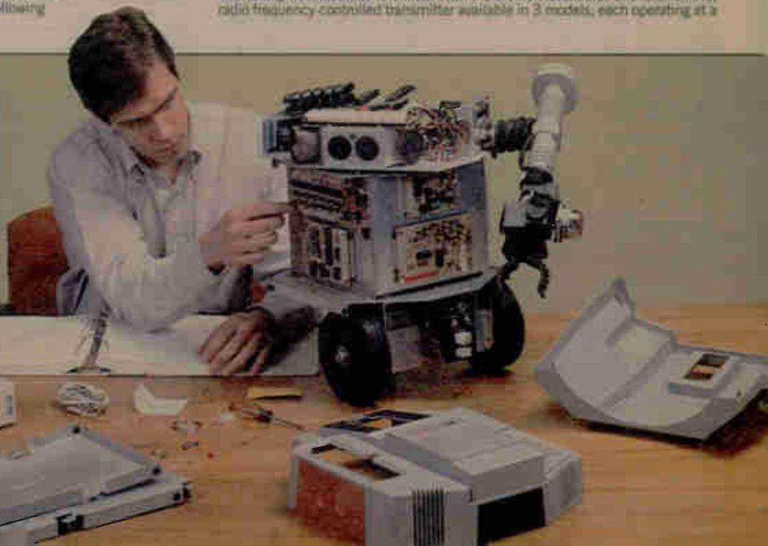
different frequency. It controls all keyboard and Teaching Pendant operations from up to 100 feet away. An RS-232 connector on this accessory also permits a computer to remotely operate the robot. Control is also provided through an optional RS-232 Interface that plugs onto the top breadboard providing a direct link between a host computer and HERO 1.
