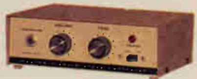
This solid-state kit takes a minimum 250 mV signal from a source (ceramic phono cartridge, monophonic AM or FM receiver, tape player, etc.) and amplifies it cleanly. Drives 8-ohm speakers to surprising sound levels! Has rear panel speaker terminals and input jack; front panel power switch with 'on' lamp, headphone jack, volume and tone controls in a 2 $\frac{5}{8}$ " H x 7 $\frac{3}{4}$ " W x 5 $\frac{1}{2}$ " D metal case. Fuse protected for 120/240 VAC.
