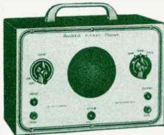
Reduces service time and greatly increases profits of any service shop. Uses crystal diode to follow signal from antenna to speaker. Locates faults immediately. Internal amplifier available for speaker testing and internal speaker available for amplifier testing. Connection for VTVM on panel allows visual tracing and gain measurements.
