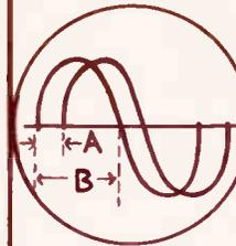
The phase shift through any stage of an amplifier is instantly shown and easily measured on oscilloscopes using a Heathkit Electronic Switch.
