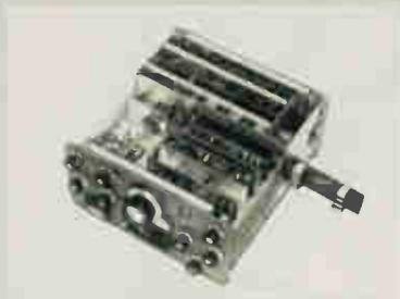
Special extender board lets you make voltage checks easily even while the receiver is operating.
