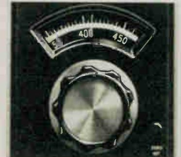
Built-in crystal calibrator lets you accurately calibrate the dial at 100 kHz intervals. Extra-large tuning knob for smooth, backlash-free tuning.
