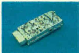
Silent All-Electronic Tuning with new combination UHF/VHF Varactor Tuner located inside the chassis where it is completely shielded.
