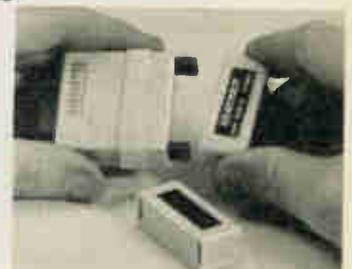
Lightweight receiver maintains the same outstanding performance with any of the 17 plug-in frequency modules. Since full-house and 8-channel systems use the same receiver, it's easy to change from 5 to 8 channels whenever you're ready.
