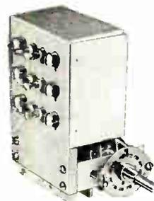
"Unit" coil and range switch turret assembly completely assembled and wired by the kit builder before installation in the chassis. Copper plated coil mounting with aluminum shield plate.
