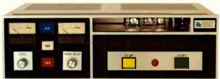
The RPD provides a third head and two separate playback systems, including amplifier, VU meter, output transformer, and output connector. This separate "Delay" system avoids loss of audio quality.
