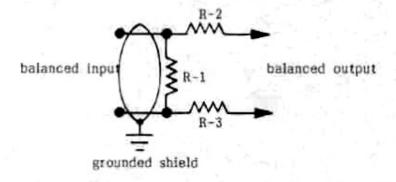
In the above example, R-1 has a value equal to the incoming line and R-2, R-3 each have 1/2 the value of the outgoing line. Balanced lines from 4 ohms to 30,000 ohms may be matched this way. At higher impedances, hum pickup may become problematic. To overcome this tendency, the balanced "line transformer" is the least expensive way to go. Telephone "repeat coils" may also be used to assure that there are no stray hums on audio lines.
