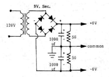
THIS SYSTEM SHOULD BE USED WITH LOW CURRENT DEVICES
