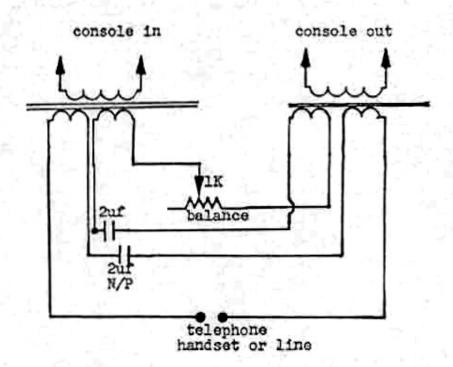
NOTE: The two transformers are identical and are usually 600 ohms value.
