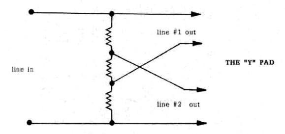
power demands. This is an impedance device and therefore should not be depended upon for power usage as its primary FUNCTION. This pad has only a 6db. loss, which is very small considering its versatility.
