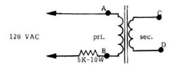
Voltage is measured on primary from point "A" to point "B" Secondary voltage is measured from point "C" to point "D"
