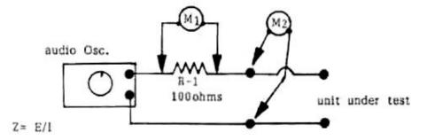
R-1 is not used if M-1 is an audio frequency AMP METER. R-1 is used in order to calculate amperage flow through the tested device by dividing the Reading of this meter by the value of "R" (100 ohms). With the current held steady at all frequencies of test (usually 20-20,000 Hz.) the impedance of the device under test may be calculated at each frequency by means of the formula: Z= E/I. M-1 gives the "I" and M-2 the "E" in the formula.
