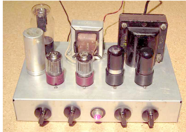
Author’s homebrew Hi-Fi audio amp made with a Lafayette chassis and parts.
