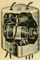
High gain composite coil used as the first detector, oscillator and first I. F. transformer, eliminates the use of one tube with no loss in efficiency. Top tuning. Factory peaked at 175 K. C. No padding condenser
