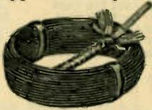
Seven strands of No. 29 wire. Cotton and rubber under waxed braid covering. Tinned. Colors: Black, Yellow, Red, Green. Shipping weight 25 ft. coil 6 oz. One piece coils.
