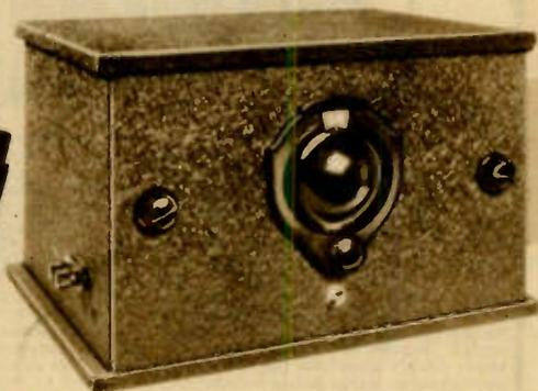
For amateur operators and advanced short-wave broadcast "fans" who do their short wave listening seriously, we offer an advanced receiver in the form of the new Lafayette A.C. set. This has a wave-length range of 14 to 115 meters, covered by low-loss plug-in coils in conjunction with a special split section variable condenser. For the sake of convenience, the power pack has been built into the set, which is therefore complete except for tubes and loud speaker.
