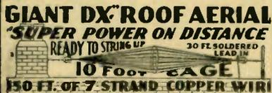
Super power on distance. Ready to string up. 25 ft. soldered lead-in. Very powerful without loss of selectivity. 10 ft. cage with 150 ft. 7-strand copper wire. Shipping weight 5 lbs.
