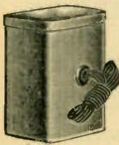
Total capacity, 12 mfd., 300 operating volts D. C. 600 V. Flash test. Red 4 mfd., Brown 3 mfd., Blue 3 mfd., Yellow 2 mfd. Black is common. Metal Container, size 5x3 3/4 x 2 1/2 ins. Made for replacement in a nationally known set. Shipping weight 4 lbs.
