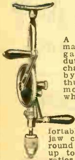
A sturdy tool made to stand the gaff of heavy duty. Two speeds changed instantly by removing a thumb nut and moving driving wheel. Closely machined gears. Large handles for firm and comfortable grip. Three jaw chuck takes all round shank drills up to 1/2 in. Gear ratios 1:3 and 1:5. Length overall 17 ins. Shpg. Wt., 8 lbs.
