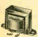
Open frame type choke. Designed to filter a current of 50 mls. Inductance of 30 henrys, 450 ohms d.c. resistance. Ideal for midjet receivers. 6 inch leads. Size, 2½x1¾x2½ in. high. Mounting centers, 3½ in. Shpg. Wt. 3 lbs. **65¢**
