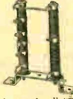
Two Truvolt type C units mounted on an insulated bracket for use with any power supply for '45 or '47 Pentode type tubes. Total resistance of 14,700 ohms, divided in seven sections to supply all "B" and "C" voltages, by means of the sliding contacts. Shpg. Wt. 3 lbs.
