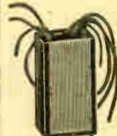
An exact duplicate of the original Crosley part No. 5315. Consisting of 1st Stage Audio and P.P. Input. No changes necessary to install this unit. Fits the chassis mounting holes. Size, 2½ x 1½ x 4¼ ins. Shpg. Wt., 4 Lbs.
