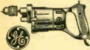
A sturdy 1/4-in. hand drill with GENERAL ELECTRIC A.C.-D.C. MOTOR and BALL THRUST BEARING in spindle. Special anti-friction bearing on armature shaft. Genuine Almond jaw geared chuck. Has toggle switch on top of pistol grip.
