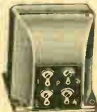
No. 1137—A matching transformer that can be used as microphone input or tube to line and in many other ways. Primary impedance combinations, 50 ohms, 100 ohms, 200 ohms; secondary impedance combinations, 2500 ohms, 5000 ohms, 10,000 ohms. Shpg. Wt. 5 lbs. List Price, \$12.00.
