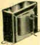
A Choke that can be used in filter circuit of power packs and amplifiers, also suitable as an output choke. D.C. resistance of 1000 ohms, C.T. Size, 2 3/4 x 1 3/4 x 2 1/4 ins. high. Mounting centers, 3 3/8 inches.
