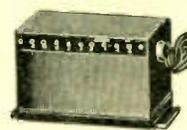
Consists of a standard Jefferson power transformer and a heavy duty choke sealed in a compact metal container. 110-120 volts, 50-60 cycle. 700 volts, high voltage at 110 mls., C. T. Size 7" long, 3 1/2" wide, 6 1/2" deep. Bottom brackets for convenient mounting. Shipping weight 19 lbs.
