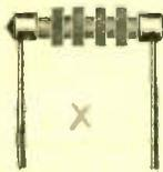
An excellent choke for use in receivers or in lowpowered transmitters. Wound in 4 sections on isolantite form. Extremely low distributed capacity. Inductance 2 1/2 millihenries; D. C. resistance 50 ohms; distributed capacity 1 mmd.; rating 125 M. A. Can be mounted in grid-leak clips or with stiff wire leads.
