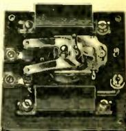
This relay is designed to be used with an adjustable mercury thermo-regulator. With this type of regulator it is possible to accurately control temperature in ovens, incubators, etc., to very close limits. Relay is designed to reduce voltage and current to be broken by instrument contacts. For example, 110 V. 60 cycle control the amperage would be approximately 12 milliamperes. Contacts will handle up to 30 amps. 110 V. A. C. Shpg. wt. 7 lbs.
