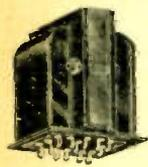
Can be used in Balkeit A3, A5, A7; Fada 16, 17, 20, 32, 50, 70, 71, 72; Crosley 804; Eveready 30 Series, and Steinite 40-A, 45-A. 2½-volt winding for 5-227s, 5-volt winding for 2-171As, 5-volt winding for 280 tube; 285/285 volt at 60 MA. 120-volt primary. Size 4½x3¼x3¼". Mounting centers 2½x2½". Soldering lugs terminate on an insulated strip. Shipping weight 7 lbs.
