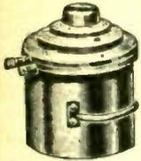
A powerful Dynamic Unit especially designed for use with trumpet type horns. Handles 20 watts continuously or 50 watts peak. Has 15 ohm voice coil and requires 6-8 volts at 1.1 amps for field excitation. Has threaded collar for attaching horn or the triple connector described below. Shpg. wt. 26 lbs.
