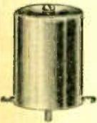
24 mh. R. F. choke, shielded, for general use short wave and broadcast receivers. Effective range extends from 600 K.C. to 20,000 K.C. distributed capacity 12.5 mmf. D. C. resistance 145 ohms. Current carrying capacity 40 M. A. Real inductance is 24.5 M. H. Fully shielded in drawn aluminum shell.  $1\frac{1}{4}$ " high,  $1\frac{1}{4}$ " diameter. Shipping weight 1 lb.
