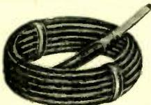
Forty strands No. 29; 14 Gauge. Layer of heavy cotton under covering of live rubber. Tinned. Ideal for heavy duty filament in transmitting apparatus. Shipping weight 25 ft., 1 lb.
