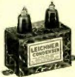
These condensers are a radical departure from conventional design in that they have high quality Flint Glass plates as the dielectric. By using flint glass only about .00291% of the power flowing through the condenser is lost. In some mica con-
