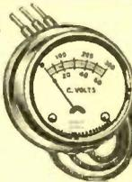
The A. C. meters are of the repulsion type and may be used with accuracy for either A. C. or D. C. testing. Not to be confused with the ordinary vane type with its restricted application. The higher reading A. C. voltmeters have over 100 ohms per volt resistance. The D. C. voltmeters are of the polarized vane solenoid type and contain resistance up to 800 ohms per volt.
