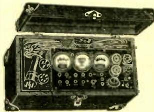
A three meter analyzer that quickly checks all voltages, plate current, etc. Charts furnished for measuring resistances to 100,000 ohms and testing condensers. Scale readings are 0-20-60-300-600 D. C. volts, 0-10-140-700 A. C. volts, 0-15-150 M. A. D. C. meter resistance 300 ohms per volt. Case has space for tools, etc. Analyzer in removable tray. Shpg. wt. 10 lbs.
