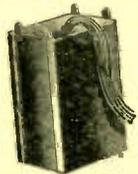
Consists of a push-pull inter-stage audio, primary 2300 ohms center-tapped, secondary 7600 ohms center-tapped. Output, push-pull audio, primary 600 ohms center-tapped, secondary, 10 ohms. Can be used with any receiver or power amplifier using p.p. pentodes in the output stage to the voice coil of a dynamic speaker. Unusually small in size, 3 3/4" high, 2x2 3/4". Metal container, completely shielded and pitched against moisture. Crimping lugs for easy wiring. Shipping weight 5 lbs.
