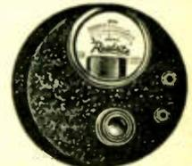
Mounted in seamless steel cases 4" in diameter. Model 500 provides direct readings of ohmages up to 10,000 and D. C. volts up to 4.5. Model 502 furnishes readings to 10,000 ohms on one scale and up to 40 ohms on second scale, for voice coils and shorted turns of IF transformers. Both are complete with a small 3 cell flashlight battery and leads. Shipping weight 2 lbs. **K11020—List \$6.50**
