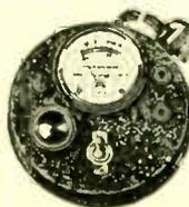
This efficient capacity meter, which should be part of the equipment of every serviceman, is used for testing paper condensers only.
