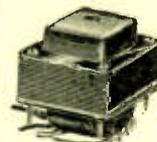
Here is a universal flush mounting type transformer, for replacement in receivers using up to 9 tubes. Equipped with leads and soldering lugs. Extra heavy windings: 2.5 V. at 8.5 amps. 2.5 V. at 3 amps. 5 V. at 2 amp. 340/340 high voltage at 90 M. A. 115 V. 50-60 cycle primary. Size 3¼x3¼x2¼", mounting centers 2½x3½". Shipping weight 8 lbs.
