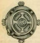
An excellent inexpensive double button carbon microphone for the Ham station or for P.A. systems used chiefly for voice reproduction. Diaphragm has gold spot contact surface. 200-ohm impedance. Frame diameter 2 1/4" Frame thickness 1/2". Screen protected diaphragm. Bright nickel finish. Shpg. wt. 1 lb.
