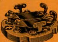
These double trimmer condensers are used to tune I.F. stages to the same frequency so that maximum signal response and sensitivity can be obtained. Have Isolantite tops, 1 1/4" in diameter for a 2" shield. Capacity range 10 mmf. minimum to 70 mmf. maximum.
