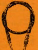
A 30" remote control cable which governs the condenser gang and the dial scale. One end has a flattened shaft, the other has connecting rod for insertion in condenser gang coupling. Part No. 6497. Shpg. wt. 1 lb.
