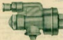
For all refrigerants except ammonia, carbon dioxide, range 20 inches vacuum to 15 lbs. pressure. Moisture proof, forged brass body. Length overall 3 1/2". Standard inlet 1/4" S.A.E. on valves. With 1/4" and 3/8" F.P.T. outlet any standard fittings may be used.
