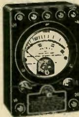
A small compact Volt-Ohmmeter with ranges of 0, 3, 30, 300, 600 volts and 1,000-100,000 ohms. Supplied with self-contained battery and 50' test leads. A control is provided to compensate for drop in battery voltage. Two toggle switches select ohmmeter ranges and change meter for volt or ohmmeter circuits. Bakelite case size 5 1/2 x 3 1/4 x 3". Shpg. wt. 3 lbs. **XJ10554**—Model 564 Volt-Ohmmeter, Type 3A. **Your Cost \$22.05**
