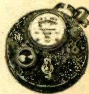
Contains rheostat, switch, test leads and plug for A. C. 60 cycle connection. Instruction furnished for testing from 10 to 400 henrys, and resistances from 40 to 100,000 ohms. Shpg. wt. 2 lbs.
