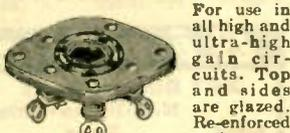
For use in all high and ultra-high gain circuits. Top and sides are glazed. Re-enforced spring contact. Size 2 1/4 x 1 1/8"; mounting centers 1 3/4".
