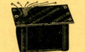
RCA Part No. 5899. Used in the 106 A. C. speaker and in the 41 A. C. and D. C. sets. Used to match a single 71A, 45 or 50 tube to a 5-15 ohm voice coil. Also contains two 1 mfd. condensers. Shpg. wt. 3 lbs.
