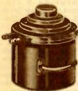
A powerful Dynamic Unit especially designed for use with trumpet type horns. Handles 20 watts continuously or 50 watts peak. Has 15 ohm voice coil and requires 6-8 volts at 1.1 amps. for field excitation. Has threaded collar for attaching horn or the triple connector described below. Shpg. wt. 26 lbs. **\$32.34**
