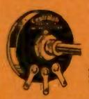
Manufactured by Centralab. Potentiometer type, 25000 ohms. Tapered for an antenna or bias. Milled shaft 1 1/2" long. Bakelite case.
