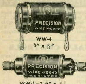
Precision wound resistors for use as meter multipliers and similar applications. Guaranteed accuracy 1%. WW-1 has ferrules with binding post terminals; resistor WW-4 has tinned solder lug terminals.
