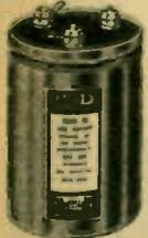
Can be mounted in upright, horizontal, or any other position without affecting operation. All provided with mtg. rings. Can is negative. Rated peak voltage 525; wkg. voltage 450v. d.c.
