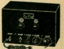
Range 50 to 30,000 kc. in six bands; all fundamentals. Dial is 25" long and is divided into 400 divisions providing accuracy of 1-10% in reading. Supplied with 11x17" calibration chart. Continuously variable output 1/2 microvolt to 2 volts. 400 cycle audio note. a.c. or d.c. (110v.) operation. Black crackle case. Shpg. wt. 15 lbs.
