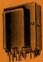
Fully shielded in metal case with crimp lugs for mounting. Primary for 110 volts, 50-60 cycles a.c. Secondaries: high voltage delivers 250/250 volts at 65 ma.; 6.3 volts at 1.5 amps. (for 3 heaters and 1 power tube); 5 volts at 2 amps.
