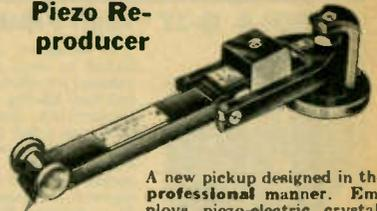
A new pickup designed in the professional manner. Employs piezo-electric crystal. Needle pressure adjustable from 1 to 3 ounces; graduated scale shows exact pressure. Excellent frequency characteristics. High impedance, may be connected directly to input grid. Cast aluminum arm with instrument black finish. 14" long, 3½" high. Shpg. wt. 8 lbs. List \$60.00
