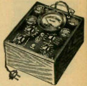
Tests all types of tubes—both glass and metal. Has 3 1/2" quality meter with a colored "Good" and "Bad" scale. Makes all short tests, cathode leakage tests and individual tests on diodes and full-wave rectifiers. Includes rectifier tube and line voltage regulator. Has only 4 sockets, is of the emission type and operates on any 100-130 volt, 60-cycle, a.c. source. No confusion, complications or calculations. New metal case, 7 1/2 x 6 3/4 x 4 3/8". Shpg. wt. 15 lbs.
