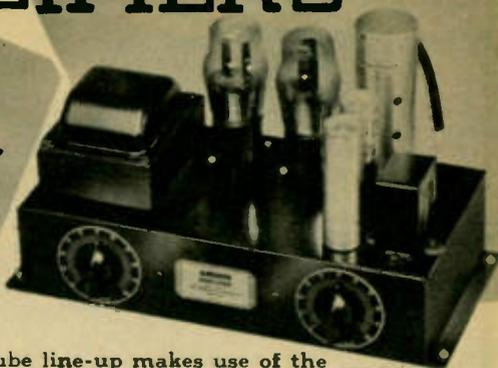
The tube line-up makes use of the new pentodes, 57 and 2A5 power output, as well as an 83 mercury-vapor rectifier. Gain is 76 db, overall. The entire unit can easily be placed in a convenient cabinet or carrying case, and used wherever A.C. is available.
