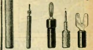
Needlepoint prods have chuck that takes standard phonograph needle which is easily replaced.
