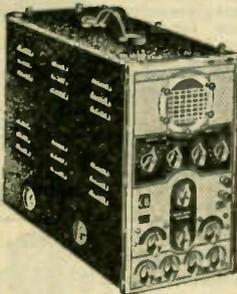
Is complete for every servicing, experimental and transmitting radio need as well as industrial application. Permits study of wave forms of frequencies at 100,000 cycles or higher. Combines in a single housing two input amplifiers, linear sweep circuit and power supply for all tubes. Employs a 906 (3") cathode-ray tube, a 57, a 2A5, an 886, an 80 and an 81.
