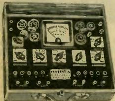
A complete servicing unit. Tests ALL tubes under load conditions—all elements for opens, leaks, shorts and NOISE; hot cathode leakage test by both neon and meter; hum test. Is double-fused. Smooth line voltage control. Free, floating filament circuit and other features guard against obsolescence. Multitester offers: 5 a.c. and d.c. voltage ranges: 5/25/125/500/1250; 4 ohm ranges: 0/100/25,000 ohms, 0-2.5/25 megohms. Ohms read as low as .05. 0-500 microamps.; 5/25/250 d.c.
