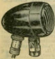
New streamlined dynamic mike. High impedance, 10,000 ohms (high permeability transformer built-in). Output level -55 db. Response  $\pm 1$  db. from 50 to 5,500 c.p.s.;  $\pm 3$  db. from 50 to 7,500 c.p.s. No pronounced peaks. Not affected by temperature changes, humidity or wind noises. Semi-directional. Streamlined case finished in black with chrome plated grill. 3 1/4" long, 2 1/4" diam. With swivel for 3/4"-27 thread, 25 feet of rubber covered cable and Amphenol connectors. Shpg. wt. 6 lbs.
