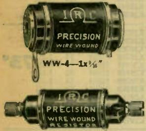
Precision wire-wound resistors designed for use as meter multiples and other applications where great accuracy is a requisite. Guaranteed accuracy 1%. These resistors are non-inductively wound. Winding is fully shielded. Type WW-1 has ferrules with binding post terminals. Resistor type WW-4 has tinned solder terminals.
