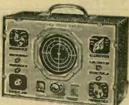
125 kc. to 60 megacycles. 5 bands on fundamentals, 125 kc.-15 mc. 4 $\frac{1}{2}$ " full-vision direct-reading dial—no charts. Output can be modulated or unmodulated. 30% modulation 400 cycles, sine wave from self-contained independent 400 cycle circuit. Attenuation in calibrated steps, 1 microvolt- $\frac{1}{2}$  volt. Provision for external sweep and wobulator for oscillography. Fully shielded. For 110/120 volts, 50/60 cycle a.c. Gray cabinet. **K21592—List \$29.35**
