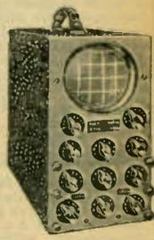
Power supplies deliver 1125 and 415 volts, assuring brilliant pattern. Size: 14x8x15 1/4". Du Mont Type 168, 5" Oscilloscope complete with all tubes, accessories and instructions. K21585—For 110 v. 50/60 cycles a.c. Shpg. wt. 35 lbs. Your Cost **\$114.17** Complete .....
