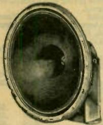
A high powered, high fidelity 12 inch speaker for p.a. use, for the better receivers, etc. Will handle 15-watts of audio power continuously. Voice coil 2 1/4" in diameter, Impedance 10 ohms at 400 c.p.s. Field resistance 2500 ohms. Overall size: 12 1/4 x 8 1/4". Furnished with transformer. Shpg. wt. 25 lbs.
