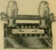
Operates on 110 volts a.c. or d.c. 600, 800 and 1000 cycles notes. For practice or modulation; outputs, 2,000 ohms at plus 10 db, 200 ohms at minus 30 db. With cord and plug. Equipped with two Bakelite terminal strips which mount screw-type binding posts. Uses two 76 tubes. 6 1/4" long, 4 1/4" wide, 1 3/4" high. Less tubes.
