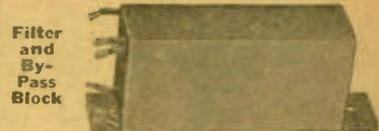
Suited for use in a.c.-d.c. midgets. Four sections: 16 and 8 mfd. at 200 volts peak, 5-5 mfd. at 35 volts peak. Color coded leads. Size:  $3x1\frac{1}{2}x1\frac{1}{2}$ "; centers  $3\frac{1}{2}$ ". Shpg. wt. 1 lb. List price \$1.75. K3202—10 For \$3.25
