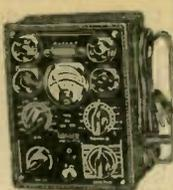
Proper load values are applied to tubes under test. The circuit is designed to indicate all inter-element shorts and leaks. Four flush-mounted sockets provide for all tubes, one 5-6 in combination to minimize panel space. Has a.c. meter for line volts adjustment. Operates on 110 volts, 60-cycle a.c. In black metal case, 5 1/2 x 7 1/8 x 4 1/8". Wt. 9 lbs.
