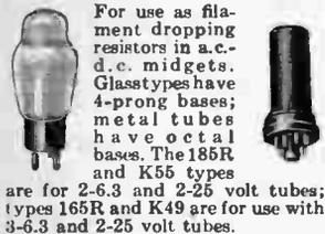
For use as filament dropping resistors in a.c.-d.c. midgests. Glasstypes have 4-prong bases; metal tubes have octal bases. The 185R and K55 types are for 2-6.3 and 2-25 volt tubes; types 165R and K49 are for use with 3-6.3 and 2-25 volt tubes.
