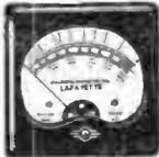
D'Arsonval moving coil type movement (50 mv.). In 3" square bakelite case requiring 2 $\frac{3}{4}$ " panel hole. With zero adjuster. Shpg. wt. 2 lbs.
