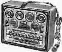
Improved push-button analyzer for plugging-in receiver socket for measuring voltage, current, resistance or capacity in any radio unit. Safeguarded against "shorts" when 2 or more buttons are pressed. Permits current and voltage measurements in same circuit at same time. Incorporates 6 sockets, including Loktal. Complete with cable, toggle latch-type plug and 7 adapters. 8 3/4 x 7 3/4", in natural finish wood case. Wt. 5 lbs. Model 504C.
