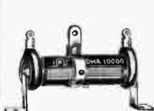
IRC wire wound variable resistors have received universal acceptance by servicemen everywhere. They dissipate heat rapidly, are built to withstand heavy overloads and have great mechanical strength. The slider feature makes them invaluable—by moving the metal contact band practically any desired range within value of the unit can be obtained. Mounting brackets with all except 10 watt units.
