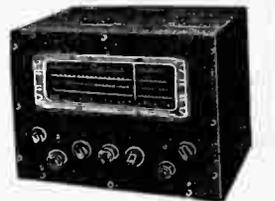
A highly efficient, low priced receiver that covers from 7.1 to 560 meters in four overlapping bands. Features: Air tuned multi-wave coil assembly, **factory wired and aligned**; slide rule dial with 9" linear scales; beat freq. osc. with pitch control and cut-out switch; Ferrocart (iron core) I.F. transformers; R.F. gain and automatic volume controls; Audio volume control; 3-gang precision condenser; 8-octal base tubes. Kit includes all parts except tubes and speaker. Diagrams furnished.
