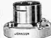
Low-absorption porcelain material base. Heavy phosphor bronze contacts, cadmium-plated, with double filament springs. Heavy nickelled brass shells.
