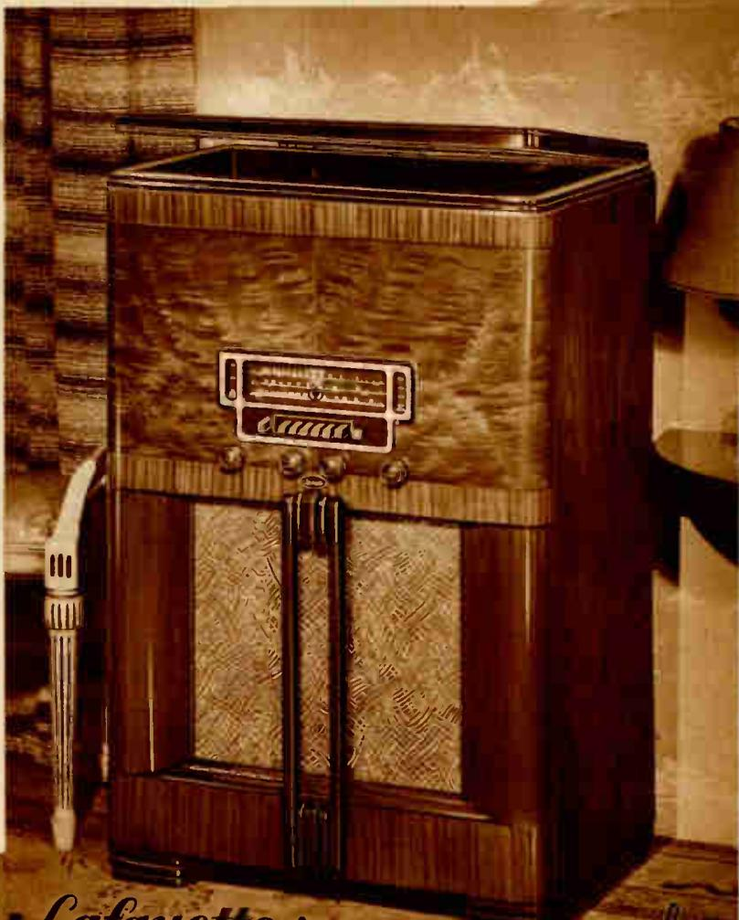
The Lafayette Custom-Built 11-Tube A.C. 3-Band Superhet is available in several different models. Chassis, speaker and tubes only (model BB-10) as illustrated on page 22; housed in the radio Console Grand Cabinet (model BB-11) as illustrated on page 22; with a Garrard Automatic Record Changer, in deluxe combination cabinet (model BB-12) shown at right; with Garrard Single Record Player (model BB-13) in combination cabinet shown at right.
