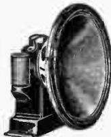
Excellent for theaters, public address systems, fine radios, phonos or wherever the finest possible performance is desired. High Fidelity models have frequency response up to 9000 c.p.s.—Standard Fidelity up to 5500 c.p.s. Power handling capacity—25 watts continuous—40 watts peak. Voice coil 8 ohms at 400 cycles. All A.C. models supplied with rectifier tube. No output transformer included. See listing at bottom of page for transformers.
