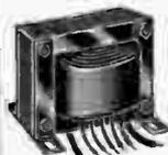
Open type with long color coded leads. Have primary, high voltage and rectifier filament windings. Will deliver full rated voltages and current efficiently. Primaries for use on 105-120 volts at 50-60 cycles a.c. Sturdy construction, will give
