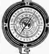
Has  $5\frac{1}{2}$ " full-vision scale and double knife-edge pointer. Glass lens. Calibrated in 3 bands: 520-1600 kc.; 1500-1600 kc.; 5.8-15.8 mc. Last scale also calibrated in meters and word descriptions. Ratio  $5\frac{1}{2}$ :1 in 180°. Has  $\frac{1}{4}$ " shaft and positive friction grip drive, 2 pilot light sockets and 6" bronze escutcheon. Takes either  $\frac{1}{4}$ " or  $\frac{3}{8}$ " shafts.
