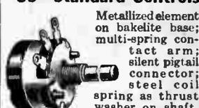
Metallized element on bakelite base; multi-spring contact arm; silent pigtail connector; steel coil spring as thrust washer on shaft. Shafts  $2\frac{1}{4}$ " long, milled.  $\frac{3}{8}$ " bushing. Taper indicated as follows: A—Uniform; B—Tone Control or Audio; C—Antenna Shunt or Audio; D—Antenna and "C" Bias; E—"C" Bias; F—Antenna and Bias; H—tapped, Tone Compensation. **Units marked with asterisk include 300 ohm bias resistor.**
