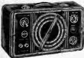
Operates on 110-120 volts 50/60 cycles a.c. Range: 100-30,000 kc. (300 to 10 meters) in 6 bands. Giant 6" dial calibrated in frequency, accurate
