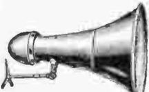
When you must throw a great deal of sound over a considerable distance—use this new Lafayette Trumpet. Constructed of heavy spun steel alloy—yet light in weight. Overall length—36". Bell diameter—24". Designed for 8" cone unit. Mounting fixture welded to trumpet. Bracket with swivel available extra.
