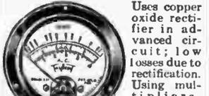
For measuring noise levels in P.A., theaters, broadcast stations, etc. Range reads up 6 and down 10 db. Zero db at 1.73 volts, 500 ohm lines, 6 milliwatts. Standard damping. Wt. 3 lbs.
