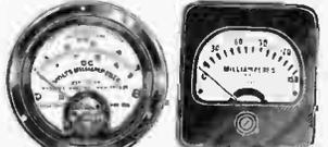
Ranges above 30 ma. are shunted and have drop of approximately 100 mv. Accuracy within 2%. Round or rectangular black bakelite cases.
