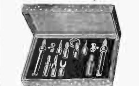
Contains 2 each—short and long banana tipped prods, alligator clip, phone tip and lug adapters, insulated banana plugs, banana jacks. Colored red and black. **\$1.15**
