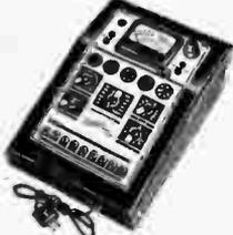
Deluxe model with 4 1/2" meter. Tests all tubes, plus ballasts, pilot lights, etc. Provision for future tube types. Smooth line voltage control; short, leakage tests. Self-contained 2-range ohmmeter, 0/10,000 and 0/1 meg. 2-range capacity tester, .001/4 and .4/16 mfd. Neon leakage indicator. Sloping panel wood case 10x15x7". For 110 volts, 50/60 cycles a.c. Complete. Shpg. wt. 20 lbs.
