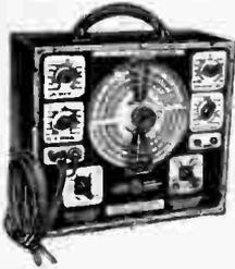
Use the Precision A.V.C. substitution system which is incorporated for simplified, precise circuit alignment. Provides bias for connection to receiver, to replace the AVC and permit alignment of circuits without AVC interference. Freq. ranges 110 KC through 72
