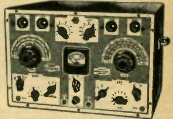
Checks a receiver from antenna to loudspeaker. Unit performs following major tests.
