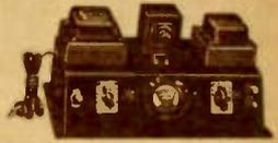
For supplying 6 volts of pure d.c. power from any 110 v., 60 cycle a.c. line. Eliminates the messy 6 v. storage battery. All employ 24 junction copper-oxide rectifiers, eliminating tube replacement.
