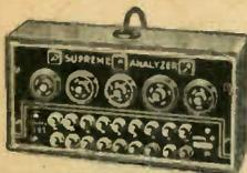
Permits connection to any multi-meter, which enables making essential tests within any receiver without removing chassis. Voltage, current and resistance measurements all made by pressing push-buttons. Six sockets, including Loktal, are incorporated. Analyzer plug replaces tube in set's socket. In Oak Carrying Case, with cable, plug adapters, etc. Shpg. wt. 8 lbs.
