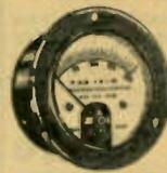
Model 311. Overall diameter 3 3/4". Bakelite case. Furnished with translucent dial scale; circular cutout in meter back for mounting pilot light socket (listed below). Entire scale becomes illuminated. Meter has D'Arsonval movement, Sapphir bearings, accurate to within 2%. zero adjustment, aluminum pointer.
