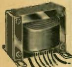
Open type with long color coded leads. Have primary, high voltage and rectifier filament windings. Will deliver full rated voltages and current efficiently. Primaries for use on 105-120 volts at 50-60 cycles a.c. Sturdy construction, will give
