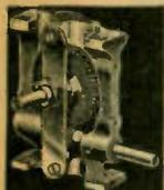
Right-angle worm drive assembly for variable condensers, etc. May be panel or base mounted. Ratio 16 to 1. Frame of cast aluminum. Employs spring-loaded split gears which eliminate back lash. Drive shaft  $\frac{1}{4}$ " diam.; geared shaft  $\frac{1}{8}$ " dia., couples to condenser by means of flexible coupling (not supplied). Excellent for transmitters and receivers. Shpg. wt. 2 lbs.
