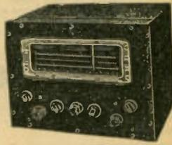
A highly efficient, low priced receiver that covers from 7.1 to 550 meters in four overlapping bands. Features: Air tuned multi-wave coil assembly, **factory wired and aligned**; slide rule dial with 9" linear scales; beat freq. osc. with pitch control and cut-out switch; Ferrocart (iron core) I.F. transformers; R.F. gain and automatic volume controls; Audio volume control; 3-gang precision condenser; 8-octal base tubes. Kit includes all parts except tubes and speaker. Diagrams furnished.
