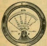
0-1 d.c. milliammeter Foundation Instruments with internal resistance of 100 ohms (1000 ohms-per-volt). Scales read: 0-10-50-250-500-1000 volts; 0-1-10-50-250 milliamperes; low ohms, .2 to 600; high ohms to 100,000. Shpg. wt. each, 3 lbs.
