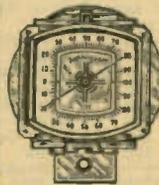
This attractive modernistic dial will dress up any receiver. Scale supplied is universal for use with either clockwise or counter-clockwise condensers. Ratio 10:1 in 360°. With 2 dial-lite sockets. For use with both  $\frac{3}{8}$ " and  $\frac{1}{4}$ " condenser shafts. No necessity for special cabinet cutout—will fit standard  $\frac{3}{8}$ " round opening. With escutcheon.
