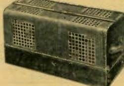
Professional type amplifier chassis and covers. Chassis is of one-piece cold-rolled steel, with reinforced corners, with ventilated covers. Finished in rippled black; cover in slate gray with polished striped chromium molding and red striped chromium handles. All covers 6" deep. (Chassis drilled for bottom covers (not supplied).)
