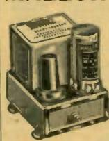
Flexible, heavy-duty vibrator power supplies designed to provide the most dependable and low cost method of obtaining "B" voltage from storage batteries. Specially designed for supplying high voltage d.c. for amplifiers, receivers and transmitters in cars, boats, etc. Features include: flexibility provided by four output voltages in 25-volt steps; high efficiency; compact. Tube type required where "B" minus cannot be at ground potential. Shpg. wt. 10 lbs.
