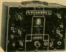
Five frequency ranges from 70 kc. to 15 megacycles; harmonics to 60 mc. PUSH-BUTTON tuning. Nine selected frequencies (the 6 most
