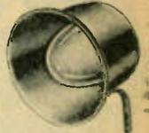
Similar to larger units listed above, this design also makes for extremely compact construction. Invaluable where the speaker must be inconspicuous. Bell—10" diam. Overall depth—8". Heavy aluminum bell. Bullet insert of Racon acoustic material. Speaker 5" power type PM. Cap. 5 watts. 6 ohms voice coil. Shpg. wt. 4 lbs.
