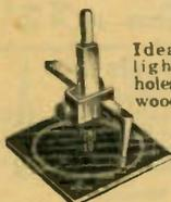
Ideal for average light work. Cuts holes in aluminum, wood, bakelite, hard rubber, etc. Shank diameter 3/8". Single set screw. Shpg. wt. 2 lbs.
