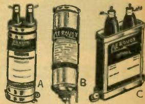
Hvyol oil filled and impregnated transmitting condensers. Hermetically sealed in metal containers. Rated capacity remains constant over a wide range of temperature (minus 30 to plus 200° Fahrenheit). Type "A" and "C" (shown at right) have universal type mounting. Type "B" is screw type with lug. Types "A" and "C" are aluminum cans—Type "B" welded steel aluminum finish. Shpg. wt. 2 lbs.
