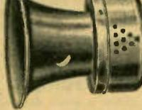
Sturdy short-flair-aluminum horns, for call and inter-office communication systems and public address installations. Finished in battleship-gray; with air vents for ventilation. Removable back makes speaker mounting simple. In two sizes, for 5" and 6" dynamics. 5" unit is 6 1/2" long; 6" is 9 1/2" long.
