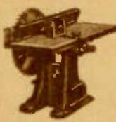
Heavy cast-iron table, 8 $\frac{1}{2}$ x11"; ground finished with vertical adjustment up to 2". Cast-iron, ground finished fence. 1-piece steel mandrel, for  $\frac{1}{4}$ " bore-24 thread accessories. High-grade bearings. Base 6 $\frac{1}{2}$ " high, designed for tool rests and guards. 1" V-type steel pulley, for  $\frac{1}{2}$ " V-belt. Handles materials up to 2" in thickness. With 6" coarse Circular saw blade. **K15355**—Shpg. wt. 12 lbs. **4.45**
