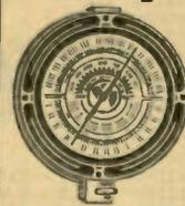
Has  $5\frac{1}{2}$ " full-vision scale and double knife-edge pointer. Glass lens. Calibrated in 3 bands: 520-1600 kc.; 1500-4600 kc.; 5.8-15.8 mc. Last scale also calibrated in meters and word descriptions. Ratio  $5\frac{1}{2}$ :1 in 180°. Has  $\frac{1}{2}$ " shaft and positive friction grip drive, 2 pilot light sockets and 6" bronze escutcheon. Takes either  $\frac{1}{4}$ " or  $\frac{3}{8}$ " shafts.
