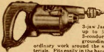
One of the finest makes of drills, for radio shop or home. Husky aluminum casings, oil-less bearings, powerful efficient motor, 3-jaw Jacobs chuck and key (for drills up to 1/4"), thumb-control switch, 3-conductor cable and plug (one for grounding). Powerful enough for all ordinary work around the shop in steel and softer materials. Fits easily in the hand. Overall length—12". Net weight 3 1/2 lbs. For 110 volts A.C. and D.C. operation.
