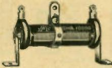
IRC wire wound variable resistors have received universal acceptance by servicemen everywhere. They dissipate heat rapidly, are built to withstand heavy overloads and have great mechanical strength. The slider feature makes them invaluable—by moving the metal contact band practically any desired range within value of the unit can be obtained. Mounting brackets with all except 10 watt units.
