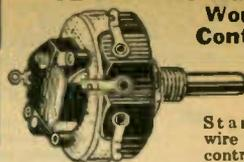
Standard wire wound controls in bakelite cases. Switch covers easily attached. Control diameter 1 1/2". Mount in 3/8" hole. 3/8" shaft extends 1 1/2". Units marked with asterisk (\*) are rheostat type; all others are potentiometers.
