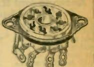
Finest hi-frequency Socket. Made with polystyrene base. Break-down voltage—12,000 volts D.C. Long contact soldering lugs. With mtg. plate Octal only. **K13170 Your Cost Each 29c**
