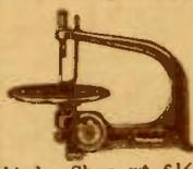
Rigid cast iron frame, with 8" dia. cast iron table tilting to 45 degrees either direction.  $\frac{1}{2}$ " driveshaft runs in cast iron bearing with adequate provision for oiling. Rocker arm and Pitman rod drive. With 2-step die-cast "V" cone-drive pulley.  $\frac{1}{2}$ " stroke; permits handling up to 1" material and cuts to center of 18" circle. Uses any 5" straight-end blade. **K14978**—Overall H. 12 $\frac{1}{2}$ ". Less motor and blade. Shpg. wt. 6 $\frac{1}{2}$  lbs. **1.49**
