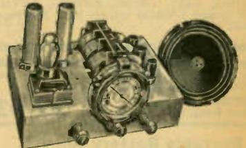
A fine 7 tube receiver that will give excellent results. The TRF circuit used is similar to that used in modern high fidelity receivers and will give excellent tone quality. Tubes used: 2—6SK7, 1—6SJ7, 1—6SC7, 2—6G6G and 1—5Y3.
