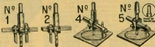
Cut holes in brass, aluminum, steel, wood, Bakelite, etc. Nos. 1, 2 and 4 cut holes from 3/8" to 4" in diam. No. 5, heavy duty type, cuts holes from 1" to 5 1/2" diam. No. 1, has extra beading cutter. All but No. 5 fit either round or square chucks either in power-driven or hand drills. Of finest heat-treated steel.
