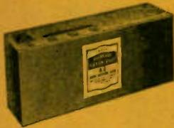
Type 748. Contains a 1½ volt "A" supply and 90 volts of "B". The latter is of layerbilt construction. Has multiple sockets for use with 1.4 volt receivers using either 3 or 4 prong plugs. Size: 15¼x4¼x6¾". Wt. 26 lbs.
