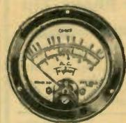
Uses copper oxide rectifier in advanced circuit; low losses due to rectification. Using multipliers, scales are: 0-15-150-750 volts a.c., or d.c., at 1000 ohms per volt, 0-1-5-15-150 d.c., ma., 0-15-150 a.c., ma., 0-1500 ohms, 0-1-5-3 megohms. Accuracy on d.c. 2%, on a.c., 5%. With D.P.D.T. switch for a.c. to d.c. change. Ideal foundation instrument for servicemen's test outfit. List \$15.00.
