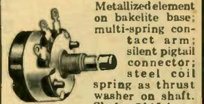
Metallized element on bakelite base; multi-spring contact arm; silent pigtail connector; steel coil spring as thrust washer on shaft. Shafts  $2\frac{1}{2}$ " long. Taper indicated as follows: A—Uniform; B—Tone Control or Audio; C—Antenna Shunt or Audio; D—Antenna and "C" Bias; E—"C" Bias; F—Antenna and Bias; H—tapped, Tone Compensation. Units marked with asterisk include 300 ohm bias resistor.
