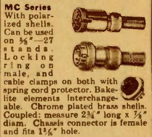
**MC Series** With polarized shells. Screw type coupling ring on male, and cable clamps on both with spring cord protector. Bakelite elements interchangeable. Chrome plated brass shells. Coupled: measure 2 3/4" long x 1 1/4" diam. Chassis connector is female and fits 1 3/8" hole. K13489—3 contact Male plug. **59¢**
