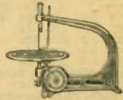
Rigid cast iron frame, with 8" dia. cast iron table that tilts to 45 degrees in either direction. 1/2" driveshaft runs in cast iron bearing with adequate provision for oiling. Rocker arm and Pitman rod drive. With 2-step die-cast "V" condrive pulley. 3/4" stroke; permits handling up to 1" material and cuts to center of 18" circle. Uses any 5" straight-end blade. **K14979—Overall height 12 1/2". Less motor and blade. Shpg. wt. 6 1/2 lbs. \$1.59**
