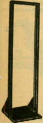
Built of 1/2" steel with spot-welded corners. Finished in ripple black. Designed for use with standard 19" long panels and are drilled for both Amateur and W. E. panel hole spacing. Bases 16" deep, 20" wide. Holes are tapped for 10-32 screws. Base is braced to insure freedom from wobble and to keep units in alignment. All heights shown below are overall dimensions.
