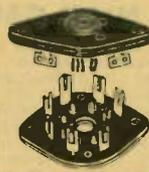
Sturdily constructed of laminated Bakelite. Cadmium-plated, self-aligning, floating one-piece contacts. Midgets have 1 1/2" centers; standards 1 1/4". No markings.
