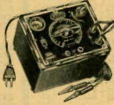
In action and works equally well with all usual capacities of mica, paper, electrolytic, and air condensers. Includes a capacity bridge with range of 10 mmfd. to 70 mmfd. Furnished complete with tubes: 1-25Z6GT, 6J5GT and a 6G5. Size: 5x6x4 $\frac{1}{2}$ " high. For operation on 110 volts 60 cycles. Shpg. wt. 6 lbs.
