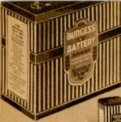
Used for many years by leading laboratories, governmental departments, commercial organizations and others demanding tops in quality. All Burgess cells are made of the best material obtainable. Each cell has a seamless drawn zinc can of 99.9% pure zinc which resists perforation. The cells are separated by moisture-resistant egg-crate partitions and a wrapping of paraffined paper. Individual cells
