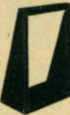
1/4" steel with black ripple finish. Mounting holes on 1 1/2" centers, tapped for 10-32 screws. Both 20" wide and 12" deep. K22102—25" high. Panel space 21x19".
