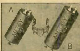
Type TCD and TCS tubulars are aluminum encased. The first are the common negative type with three terminals. The TCS tubulars are the separate section type with four terminals and can replace the common negative, common positive, or separate section capacitors. All use solder lug terminals and Mallory type TH mounting clips.
