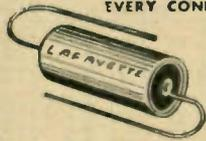
For general replacement service, extremely durable and very compact. Have high insulation resistance. Molded in extra hard, non-inflammable plastic, resistant to moisture, high temperature and shock. Extra strong copper weld leads eliminate breakage during installation. Temperature range -40° to 90° C. Made by a leading condenser manufacturer.
