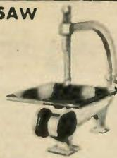
Standard duty jig saw for shop and handyman. Throat depth 12". Table 8 1/2" x 8 1/2". Stroke is 9/16". Uses 6" or 6 1/2" blade up to 3/16" wide. Self-lubricating bronze bushings. 16" height x 17 1/2" long. 3" pulley. Shpg. wt., 14 lbs.
