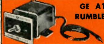
Suppresses turntable rumble and unwanted signals below 50 cycles and protects speaker from harmful sub-audio surges. Minimizes low frequency distortion. Cutoff 12 db per octave below 50 cps. No power supply required. Has standard phono input jack and 19" output lead with phono plug, on-off switch. Size: 2" H x 2 1/4" W x 3 1/4" D, with convenient mounting bracket. Shpg. wt., 1 1/2 lbs.
