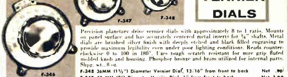
Precision planetary drive vernier dials with approximately 8 to 1 ratio. Mounts on panel surface and has accurately centered metal inserts for 1/8" shafts. Metal dials are brushed silver finish with deeply etched and black filled engraving to provide maximum legibility even under poor lighting conditions. Reads counter-clockwise 0 to 100 in 180°. Uses tough scratch resistant for sure grip fluted molded knob and housing. Phosphor bronze and brass utilized for internal parts. Shpg. wt., 8 oz.
