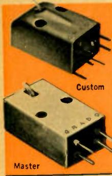
Grado Custom Features wide linear frequency response of 10-24,000 cycles. Output 7 mv per channel. Because of its high compliance, a 3 gram tracking force is recommended when used in high quality tonearms. Input impedance can be of any value above 5,000 ohms. Channel separation in excess of 20 db. Designed for use in record changers as well as tonearms. Shpg. wt., 5 oz.
