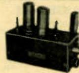
Ideal unit where space is at a premium; for mobile and home. Requires 1/2 amp of 6.3 V and 8 ma. at 100 V DC. Designed to use the broadcast band (550 kc to 1550 kc) of any receiver for tuning with a range of 1 mc. Stable operation provided by crystal-controlled oscillators. Chassis only 5" x 2 1/4" x 2 1/4" exclusive of tubes and crystal. Shpg. wt., 3 lbs.
