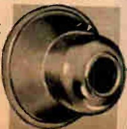
Ideal for use with tweeter and crossover networks to make up a 2- or 3-way system. This 8" mid-range speaker is capable of producing undistorted response down to 350 cps, the crossover frequency. Back is enclosed. Power handling capacity: 25 watts. Frequency response 350-13,500 cycles. Recommended to crossover at 5000 cycles to a tweeter. Cone resonance 150 cycles. Impedance: 8 ohms. Shpg. wt., 4 lbs.
