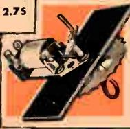
A sturdy 2 arm self-neutralizing escapement. Completely wired (not a kit). Converts electrical impulses from remote control receiver to mechanical motion for varying movement of plane, boat, or car. Four 90° rotations — two by armature activation, two by neutralization. Has ratchet governor for maintaining foolproof rotating speed. Weighs only 7/8 oz. Size: 1-3/8" L x 2" W overall. Shpg. wt., 5 oz.
