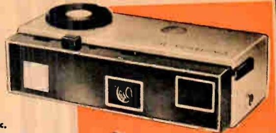
Combined film and shutter wind and instant 24-exposure clip loading. The lens is a Yashinon 25mm f/3.5 with click stop to f/16. The metal shutter has speeds from 1/25 to 1/200 sec. plus B and T, and built-in synchronization. Other features are zero reset exposure counter cable release and tripod sockets. Takes 24 B&W or color shots on 16mm perforated or unperforated film. Slides can be used on standard projectors. Make sharp, clear full sized prints. Shpg. wt., 1 lb. F-528 2.00 Down Net 27.95
