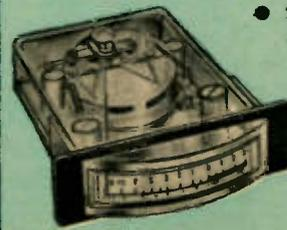
Precision D'Arsonval meters with 2% or better full scale accuracy. Front panel dimension is 3 3/4" x 1". Overall depth is 3 3/4" behind panel including terminals. Zero adjust screw. Shpg. wt., 1/4 lbs.
