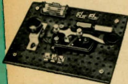
For those interested in mastering the international code, an audio tone oscillator is essential. The circuit of this transistorized feedback oscillator has the simplicity of the neon glow, the signal strength of the vacuum tube, and requires only two penlite cells for weeks of service. It may be used for solo practice, or two may send and receive with the same unit. Kit comes complete with Transistor, Telegraph Key, Resistor, Condenser, Masonite Board, etc., and Schematic Diagram. Net 1.18
