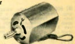
For replacement or initial motorizing of sewing machines. Powerful enough for fans-blowers-dental and jewelers lathes-hobby tools-displays. 5000 RPM full load speed, 15,000 RPM no load speed. CCW rotation facing shaft end. Cast housing 4 1/2" long, less shaft x 2 1/2x2 3/4" W. Two tapped 10-32 mtg. holes on 2 1/4" centers. 1/2" fluted shaft, 3/4" long. 12" cord lead. Fan cooled, permanent oilite bearings. Operates on 110. 120 Volts AC or DC. Shpg. wt., 2 1/2 lbs. MS-843 Net 4.95
