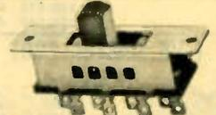
4 Position Slide Switch: Compact 4 position 2 pole slide switch. Positive snap action. Silvered contacts. Measures  $1\frac{1}{8}$ " x  $\frac{7}{8}$ " x  $\frac{1}{2}$ " overall. Mtg. centers  $1\frac{1}{8}$ ". Mtg. holes tapped for 4/40 screw. Imported
