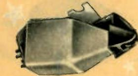
A completely mu-metal shielded stereo cartridge which has the high compliance and ruggedness demanded by all types of automatic turntables and changers. Combines high output of 10 mv per channel with extremely low signal-to-noise ratio. Freq. response:  $\pm 2$  db. from 20 to 20,000 cps.; Interchannel isolation 35 db; Tracking force 2 to 5 grams. Complete with .7 mil diamond stylus. Mounts on  $\frac{1}{4}$ " to  $\frac{1}{2}$ " centers. Shpg. wt., 7 oz.
