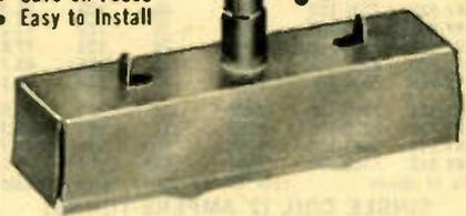
Prevent overload, and possible damage, to radios, TV, power tools, etc. This reset, thermal switch circuit breaker opens at 2.5 amps. No need to replace fuses, no fumbling in the dark—just press the button to reset the circuit. Easy to install; safest to operate. For 110-120 volts. Size: 2¾" L x ¾" D.
