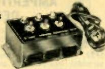
Switchable power outlet box for wall or bench mounting. Three individually controlled outlets, each with its own indicator light. Measures 4x2½x1½". Equipped with 3 polarized receptacles, 3 toggle switches, 3 indicator lights, 6 ft. line cord. Rated 5 amps at 125 volts AC/DC. Shpg. wt., 1 lb. Imported.
