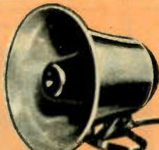
An excellent general purpose paging speaker of amazingly compact size. Ideal for portable PA systems, parties, etc. Long throw projection of 90° dispersion offers maximum speech intelligibility in high noise areas. Compact size enables it to be mounted anywhere in almost any position. Frequency response 400-12,000 CPS. Impedance 8 ohms. Power handling capacity 5 watts, 8 watts maximum. Complete with mounting bracket, 2-conductor cable. Horn diameter 5 1/4", Depth 4 3/4". Imported. Net 7.95
