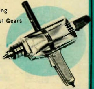
An outstanding value featuring a universal series wound motor that won't burn out. Top handle and 2-position rear handle are removable. Top quality construction with precision hobbled steel gears. 1/2" capacity in steel, 2" in wood. No-load speed 600 rpm; full load 400 rpm. AC-DC momentary contact switch with locking pin; special alloy self-oiling bronze bearings. Lustrous hi-polish finish with rich black crackle trim. Overall length 14 1/2". Shpg. wt., 12 lbs.
