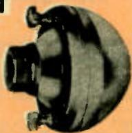
Hermetically sealed weatherproof driver unit. Delivers 25 watts of power. Perfect for any location where high volume with low distortion is desired. The PA-57 will fit any trumpet or projector of your choice without modification. The wide-range frequency response of 120-7,100 cps assures excellent reproduction of music and speech. 16 Ohm impedance matches all amplifiers. Size 4" Diameter, 3-5/8" depth. Shpg. wt., 3 3/4 lbs. Net 9.85
