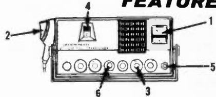
1. Illuminated Meter Indicates Relative RF Output Power, "S" reading, and Modulation
