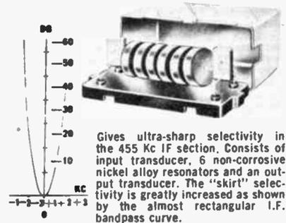
Gives ultra-sharp selectivity in the 455 Kc IF section. Consists of input transducer, 6 non-corrosive nickel alloy resonators and an output transducer. The "skirt" selectivity is greatly increased as shown by the almost rectangular I.F. bandpass curve.
