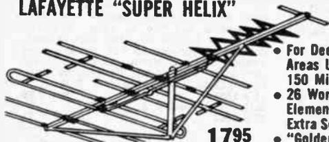
Extra-high sensitivity for crisp, clear, snow-free picture in B/W or color, out in deep fringes. Triple-driven collector system combines straight and folded dipole sections into single co-active antenna for Yagi-quality performance. High front-to-back ratios of up to 22 db on low band and up to 28 db on high band screen out ghosts. Entire 1" square boom rigidized by two 1" tubular supports. Less mast and 300-ohm twin line. Shpg. wt., 10 lbs.
