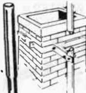
All the items for simple installation. Your choice of an all angle roof mount or chimney mount—lightning arrester—75 feet of 300 ohm twin lead—screw eyes—mast stand offs and 5 ft. 1¼" O.D. steel mast. Shpg. wt., 7 lbs.
