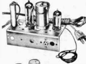
Have fun making announcements and broadcasting music through your own radio — with this broadcaster. Simply connect high impedance microphone or phono pickup to broadcaster and tune in broadcaster on radio. No wiring between the broadcaster and radio set. Pretuned to 1600 on radio dial but easily retuned. With 12BE6 and 35W4 tubes, phono jack, 2 feet of antenna, schematic and line cord. Completely wired. Chassis size: 4x2". For 110-125V AC/DC operation. Shpg. wt., 2 lbs.
