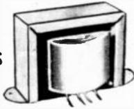
Here is an outstanding value in the most popular transistor output transformer for 10 to 11 ohm speakers. Rated power is 150 milliwatts. Primary impedance is 400 ohms, center-tapped and secondary 11 ohms. DC resistance of primary is 20 ohms and secondary .9 ohms. Size:  $\frac{3}{4} \times \frac{3}{8}$ ". Shpg. wt., 4 ozs. Imported
