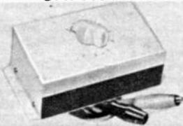
A must for the serviceman, experimenter or student. Fast accurate selection of any one of 9 capacitor values from .0001 to 22 MFD. Condensers are porcelain cased tubular type impervious to moisture and are rated at
