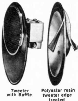
**Eccentric Tweeter Mounting & Unique Elliptical Baffle Completely Eliminates Interaction Between Woofer & Tweeter**
