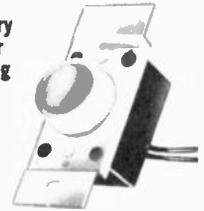
Complete variable control from off to 50% (normal dimming range), then instant switch-over to full bright. Fits into standard single gang wall box and uses same two wires as regular wall switch. Any standard wall plate can be used because knob is large enough to cover slot. Furnished with ivory plastic knob having brass-finish insert. For 120 volts, 60 cps AC with incandescent bulbs only, up to 600 watts. Size: 1 1/2" W x 2 1/2" H x 1 1/2" D. Shpg. wt., 1 lb.
