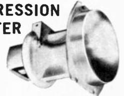
This unit offers amazing clarity and brilliance of sound. Built-in basing plug insures uniform sound output. Low end cut-off 1500 cycles; high range extends to 20,000 cycles. Handles up to 20 watts of power. Recommended crossover frequency 2500 cycles or higher. Dimensions: 5 1/4" long, mounts in 3 1/8" dia. hole. Impedance 16 ohms. Imported. Shpg. wt., 2 lbs.
