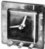
Automatically turns on radios—TV sets—etc.—at any preset time in a 12 hour period. "Sleep-Switch" allows up to 60 minutes of continuous run prior to "shut-off." Built in signal alarm. All controls on front. On-off-auto, 0 to 60 sleep switch, alarm set and time set. Gold finish dial—black lettering. 3½" square bezel, 1¾" deep. SPST rated 15 amps at 115 volts; 1650 watt load capacity. For 110-120V. 60 cy. AC only. Shpg. wt., 2 lbs.
