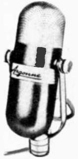
Omni-directional microphone has a swirl ridged aluminum diaphragm completely sealed and gasketed against high humidity and temperature conditions, for a wide variety of applications. The 360° stirred-up shaped bracket provides for mounting with any  $\frac{3}{8}$ "-27 thread stand. Finished in an attractive gunmetal grey with 4 $\frac{1}{2}$ " shielded cable. Shpg. wt., 1 lb. Imported
