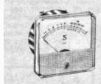
A quality "S" meter (basic 1 ma, 2 jewel movement) designed to replace many "S" meters used in communications receivers. Clear plastic front measures 2 3/8" square and meter fits standard 2 1/8" round hole. Perfect for the experimenter and amateur. Complete with mounting screws, instructions for installation and use. For 6 volt or 12 volt operation. Zero adjustment control on front panel. Imported. Shpg. wt., 1 lb.
