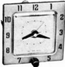
Genuine Telechron mechanism. Complete 12 hour movement. Can be set to turn on any radio, TV or similar electrical appliance at any preset time. Gold finish dial—black lettering. Timer sets from rear. On-off-auto switch in front. Size 3½" square, 1¾" deep. Set shaft extends 5½" to rear. SPST switch, rated 15 amps at 115 volts. For 110-120V, 60 cy. AC only. Shpg. wt., 2 lbs.
