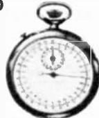
Designed for close timing. Large hand registers 1/10 of a second, up to 30 seconds; small hand reads minutes, up to 15. Start, stop, and continue from crown; instant zero. 1 jewel movement. Chromium plated case. Shpg. wt., 8 oz. Imported.
