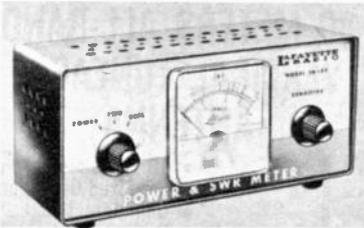
Highly accurate SWR and direct power readings up to 50Mc. The unit may be permanently inserted in the transmission line for SWR and relative power monitoring. For 52 or 75 ohm lines. Insertion loss is negligible. Meter has 50  $\mu$ a movement; calibrated directly in watts from 0.15 and in SWR from 1 to 10 IF (reads infinity at full scale) . . . Housed in an attractive grey metal cabinet, 3 1/4" x 7 1/4" x 2 3/8". Sits on 4 rubber feet. Imported.
