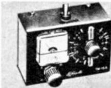
A miniature wavemeter for checking transmitter output. Determines relative strength of fundamental frequency and any harmonic or parasitic radiation. Complete and self-contained, requires no power. Telescoping antenna is included. Tunes 1.6 to 150 mc in four calibrated bands. Only 3 1/4" x 2 1/4" x 1 1/2" D. Antenna is 10 3/4" extended. 3 1/4" telescoped, is fitted with a banana plug and is removable. Total shpg. wt., 8 oz. Imported.
