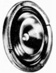
Low-cost, 3-way, full-range speaker with 3 diaphragms performing as woofer, mid-range and tweeter. Its small size, only 2" deep, makes it excellent for use in a wide variety of space-saving applications. Frequency response, 75-12,000 cps. Power handling capacity, 3 watts of program material. Impedance, 8 ohms. Shpg. wt., 2 1/2 lbs. Imported.
