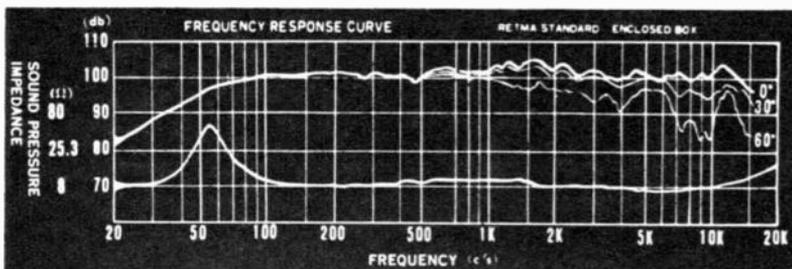
■ 20 TO 20,000 CPS (40 TO 16,000 CPS  $\pm$  3 DB) ■ HIGH EFFICIENCY ■ HIGH EXCURSION WOOFER WITH UNIQUE "CONICAL STIFFENER" ■ HANDLES HEAVY BASS PASSAGES WITHOUT "DOUBLING"
