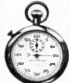
Second hand registers 1/5 of a second and completes turn in 60 seconds. Small hand indicates up to 30 minutes. Side slide starts and stops hands. Fast resetting dependable 7-jewel movement. Shpg. wt., 8 oz. Imported.
