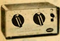
Improves receiver reception. Covers 6 through 160 meter amateur bands continuously. Uses 2 6DS4 Nuvistors in a cascode circuit for greater receiver gain and extremely low noise figure of 1.8 to 3.5 db. Also improves image and spurious rejection. Controls: 4-position range switch (1.8 to 54 MC); Antenna Tuning Control, and 3 position switch for On, off and standby. Power may be taken from receiver. Size: 5"x3"x3" D. Shpg. wt., 2 lbs.
