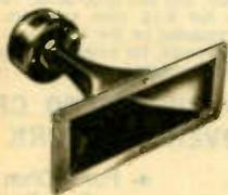
High-efficiency, wide-angle compression horn-type tweeter. Built-in pre-wired electrical crossover at 2,000 cps. Low end cut-off 2,000 cycles; high range extends to 18,000 cycles. Handles up to 30 watts of power. Constructed of aluminum, die-cast under high pressure for lasting alignment with baked-on lacquer finish. Voice coil diameter,  $\frac{3}{4}$ "; magnet weight, 1.4 oz.; impedance 8 ohms, 7 $\frac{1}{4}$ " L, 3" W, 6 $\frac{1}{4}$ " D. Shpg. wt., 1 $\frac{3}{4}$  lbs.
