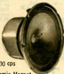
Capable of reproducing virtually undistorted sound from 350 to 14,000 cps, the recommended crossover frequencies are at 350 cps and 5,000 cps. Power handling capacity: 25 watts. Cone Resonance: 150 cps. Impedance: 8 ohms. 10 oz. ceramic magnet. Voice coil diameter: 1". Plated steel frame finished in brown baked enamel. Has 4-way binding posts. Shpg. wt., 4 $\frac{1}{2}$  lbs.
