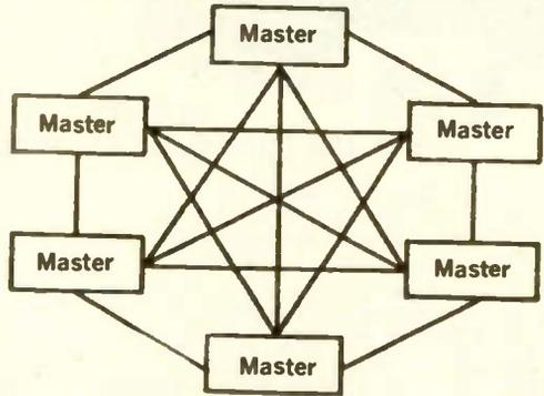
All-Master Intercom System incorporates up to six separate master stations enabling 3 private conversations or a 6-station conference to be held. Utilizes a three-position switch for listening, momentary talking, or Stand by; and a five-station selector-call switch.
