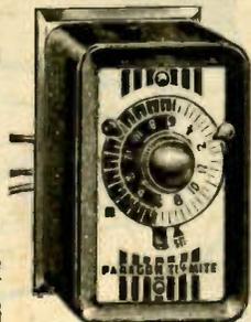
A compact time control ideal for window displays, night lights, yard lights, etc. Provides one on-off operation per day with minimum setting of two hours. Has manual trip lever. 24-hour dial is divided into 30 minute segments for easy, accurate setting. Fits over a U.S. standard single gang handy box. Size: 4½Hx2¾Wx3¼"D. Capacity: 15 amp. non-Ind., 1800W. 1 HP. 12 amps, full load. For 120 v., 60 cycles. UL and CSA approved. Shpg. wt., 1½ lbs.
