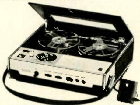
Small 6½ inch size permits operation wherever you go. Tape pack convenience lets you flip tracks without threading and record up to 32 minutes. Features built-in microphone, separate record and playback heads, 2¼ inch dynamic speaker, record level VU and speed meter, variable speed control, and end of tape cut-off. Power supplied from penlight batteries or optional external AC adapter. Size: 6½Lx 3¾Hx1½"W. Shpg. wt., 4 lbs.
