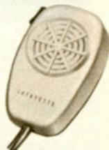
The perfect companion microphone to the "Tiny Mite" mobile PA amplifier above. Features a high impact styrol case, hang-up clip and flexible single conductor shielded cable. Omnidirectional pattern mike has output impedance of 300 ohms and output level of -73 db at 1000 cps. Frequency Response: 300-2500 cps. Grey and black case, with push-to-talk switch. Imported. Shpg. wt., 1 lb.
