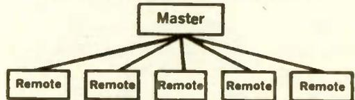
Master-to-Remote Intercom System enables master station to communicate with up to five remotes either separately or in a six-station conference. Master's 5-station selector-call switch permits private or non-private conversations. Calls may be originated by remote stations as well as master.
