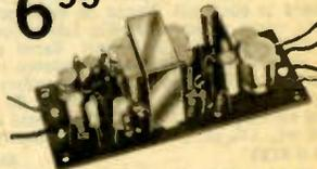
Perfect for use with tuners, test equipment or as a phono amplifier, tape recorder amplifier, PA amplifier, and telephone pick-up amplifier, etc. Requires one 9 volt battery and is readily chassis mounted. Size: 4 7/8x1 1/2x2 1/4"W. Imported. Shpg. wt., 12 oz.
