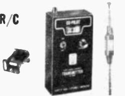
Three transistor crystal controlled audio tone transmitter operates on 27 megacycles with single 9 volt battery. Features 11-section collapsible center loaded antenna and variable output tuning. Built-in meter monitors battery current. Microswitch transmitting key actuates 100% modulated 550 cycle tone with 3/8 mile range when used with 99 D 9106 R/C receiver shown below. Black anodized aluminum case, 5 1/2 x 3 3/4 x 1 1/8". Imported. Shpg. wt., 2 lbs.
