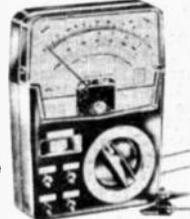
40 µA. D'Arsonval meter movement permits a high input resistance on all ranges. Rugged high impact plastic case. Ranges (DC Volts): 0-3, 30, 60, 300, 600, 3000V; AC Volts: 0-6, 60, 120, 1200V. DC Current: 0-60 µA, 0-12, 0-300 mA. Resistance: 0-60K, 0-6 megohms. Decibels: —30 to +63 db. Audio output jack. With test leads and 1½" battery. Size: 3¼x4¼x1½". Imported. Shpg. wt., 1 lb.
