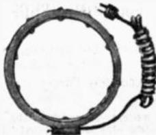
Sharpens color reception through demagnetization of the picture tube. Simply turn on the set, plug in the purifier, and with switch depressed rotate unit in front of the TV screen. Use regularly to keep your color reception sharp and clear. Save yourself dollars by degaussing your own color TV set. Supplied with line cord and plug. Convenient clip for hanging on back of set when not in use. Imported.
