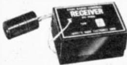
Operated with other units or as a companion to the 99 D 9105 transmitter above this 4 transistor receiver audio tones between 400 and 1000 cycles. Sensitive relay allows use of all types of escapements or single channel servos. Operates on single 9 volt battery. Lightweight (less than 2 oz.); compact (1 1/4 x 2 1/4 x 1 1/4"). Black anodized case with prewired plug. Complete with battery connector, switch, tuning wand and easy-to-follow instructions. Shpg. wt., 1 lb. Imported.
