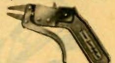
Specially designed as a multiple-service tool for small assembly work; picks up and securely holds small parts for soldering or other operations. By pushing the locking key forward, the jaws are automatically locked. Ruggedly constructed with case-hardened steel jaws. Overall length is 5 1/8".
