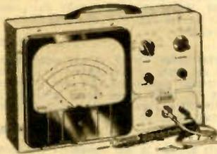
Deluxe peak-to-peak VTVM for all TV/FM/AM servicing. Features big 7 1/2" meter in "can't burn out" circuit. Has zero center scale, 1% multiplier resistors and "Uni-probe" for all measurement functions. Ranges: p-p volts, 0-4-14-42-140-420-1400-4200 v.; DC/RMS volts, 0-1.5-5-15-50-150-500-1500 v. Response, 30 cps to 3 mc. Resistance, 0.2 ohms to 1000 megohms in 7 non-skip ranges. Size: 8 1/2 x 13 x 5". For 105-125 v. 50/60 cycles AC. Shpg. wt., 9 lbs.
