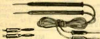
Standard test leads furnished with plastic prods and pin plugs which withstands chipping or breaking. Extra flexible kinkless vinyl covered 60" red and black leads. Prods are red and black. 4" long x 3/8" diameter. Supplied in pair of one red and one black. Available with either pin or banana plugs. Shpg. wt., 8 oz. Imported.
