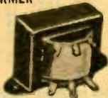
70 volt line-to-voice coil matching transformer. Primary tapped 10, 5, 2.5, 1.25 and .625 watts. Secondary tapped 5, 8 and 16 ohms. Size: 2x1 1/2". Mtg. Centers 2 3/8". Shpg. wt., 1 lb. 99 H 6284 ..... 1.49
