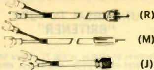
Low loss, RG-59U 72 ohm white cable. Completely assembled. 2 spade lugs on one side, choice of plug on other side fig. (R) RCA, (M) Motorola, (J) Jerrold.
