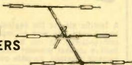
Three element beam providing up to 8 db gain on the 10, 15 and 20 meter bands. Trap design provides broadband performance and stability—beam easily handles a full kilowatt of AM signal. 25 db front-to-back ratio, SWR 1.1/1, or less, at resonance. Beam length 14 ft., element length 28 ft. Shpg. wt., 53 lbs. 40 H 5802WX \$6 monthly Net 120.99
