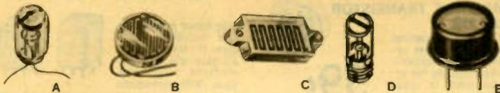
**PHOTO CONDUCTIVE CELLS.** Conductivity varies with intensity of light. All rated at 20 ma at 200 volts. Wave length 4000 to 8000 angstroms. Resistance at 0 ft. candle is 10 meg for type A, 5 meg for type B. Other chart ratings approx.  $\pm 50\%$ . Imported.
