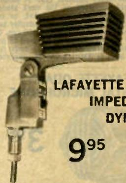
A fine quality general purpose dynamic microphone. Dual impedance selectable at cable end: high (50K ohms) or low (600 ohms) Frequency response 100-10,000 cps with high impedance. Output of —58 db. Omnidirectional pickup pattern of 325°. Has on-off slide switch. Die cast, chrome plated case. Mike case measures 5"Lx2"Hx2". Complete with 20 ft. detachable cable with mike connector. For all standard ¾"-27 stands. Imported. Shpg. wt., 3 lbs. **99 N 4581** Net 9.95
