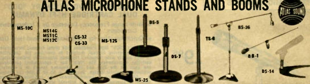
**Model MS-10C Full Grip Mike Stand.** Economical mike stand featuring "Full-Grip" clutch mechanism for fast quiet adjustments without slipping and wear. Functionally designed base assures maximum stability and includes self-leveling, shock-absorbing pads plus 3 "anti-tip" points. Full chrome plated tube assembly. Terminates in a  $\frac{3}{8}$ "-27 thread. Base dia. 10", finished in gray shrivel. Height adj., 35 to 63". Shpg. wt., 10 lbs.
