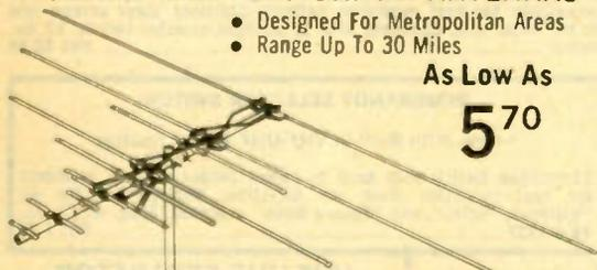
Model B-85 9 element "CROMA-FLEX". Has the high gain, high front-to-back ratio and accurate impedance match needed to pull in sharp, clear, black and white and color pictures. Features a series-fed UHF Intermixed design. A single transmission line from the antenna delivers VHF, UHF plus FM. Factory preassembled and constructed of extra heavy gauge anodized aluminum.
