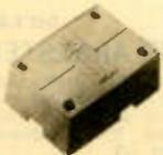
MODEL A-102U/V. An efficient coupler for all UHF/VHF Channels 2-83 plus FM. Splits signal from single down lead into 2 TV sets each having a single VHF/UHF input. Low loss design makes it ideal for fringe area use. Excellent isolation between sets prevents interaction. Patented stainless steel screws are used for rapid secure installation with 300-ohm twin lead. Sturdy, non-breakable plastic case. Shpg. wt., 1/2 lb. 18 H 1832 Net 2.20
