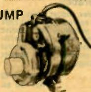
It's the all-new Delron aluminum pump for underwater use. Guaranteed not to corrode or rust; hermetically sealed motor. Circulates and dispenses water and mild acid solutions, for use in fountains, beverage dispensers, aquariums, photo developing, air conditioning, etc. Gallons per hour delivery: 240 @ 1 ft.; 180 @ 3 ft.; 125 @ 5 ft.; shut off @ 12 ft. Outlet ¾"; inlet ½" pipe O.D.; height 4½"; depth 4¼" 6 ft. safety cord. 115VAC, 60cps, AC. 49 watts load; .67 amps load. Shpg. wt., 3¼ lbs.
