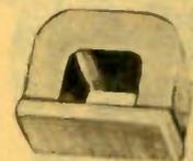
Made of Alcomax—a material with 12 times the magnetic energy of tungsten steel. Designed for efficient performance/weight ratio—will lift up to 50 times its own weight. Horseshoe shape with plated keeper. Ideal for such applications as magnetic clutch, work holding, etc. Size 1 1/2 H x 1 1/2 D x 1 3/4 W. Distance between poles is 7/8". Imported from England.
