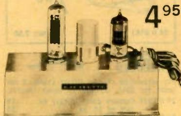
Have fun making announcements and broadcasting music through your own radio—with this broadcaster. Simply connect high impedance microphone or phono pickup to broadcaster and tune in broadcaster on radio. No wiring between the broadcaster and radio set. Pretuned to 1600 on radio dial but easily retuned. With 12BE6 and 35W4 tubes, phono jack, 2 feet of antenna, schematic and line cord. Completely wired. Chassis size: 4x2". For 110-125V AC/DC operation. Shpg. wt., 2 lbs.
