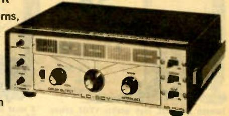
Portable, easy to use, a mighty midget, yet a giant in performance. All the patterns... crosshatch, individual vertical and horizontal lines, and adjustable white dots at the flick of a switch. 14 horizontal and 10 vertical lines, Interlace control stops dot bounce. Uses standard RCA licensed patterns. Quick warm up time. Solid State design with batteries provides patterns instantly. Rugged
