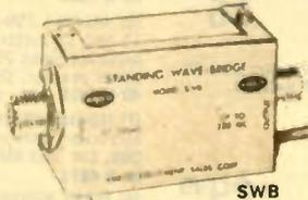
Inductive bridge that is continually left in the line. Reads SWR's from 1.8 Mc. to 225 Mc. Handles 1000W. Has negligible insertion loss. Contains two SO-239 UHF connectors. Size  $2\frac{1}{4} \times 1\frac{1}{4} \times 4\frac{1}{2}$ ". 40 H 1041 Shpg. wt., 2 lbs. .... Net 9.95
