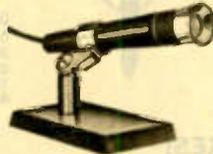
Recommended for all high quality recorders and particularly solid-state units. Has a wide frequency response of 80-15,000 cps. High impedance (10K ohms) with an output of —65 db. Die cast satin-black body with aluminum trim. Slim tapering design. May be hand-held, used on desk stand supplied or mounted in any 3/8"-27 stand. Black stand with aluminum trim. Mike is 5 1/2" x 1" dia. with 8 ft. attached cord and plug. Stand is 4 1/2 x 2 1/2". Imported. Shpg. wt., 2 lbs.
