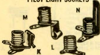
Cadmium plated brackets with tinned brass lugs. Bayonet type with coil spring construction for positive contact. For miniature screw, bayonet, and candelabra base. Threaded jewel assemblies may be used with these sockets to provide panel indicators, and are listed above. Av. shpg. wt., 2 oz.
