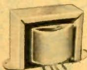
Economically priced popular transistor output transformer for 10 to 11 ohm speakers. Rated power is 150 milliwatts. Primary impedance is 400 ohms, center-tapped and secondary 11 ohms. DC resistance of primary is 20 ohms and secondary .9 ohms. Size:  $\frac{3}{4} \times \frac{3}{4}$ ". Shpg. wt., 4 oz. Imported. 99 H 6209 Net .89
