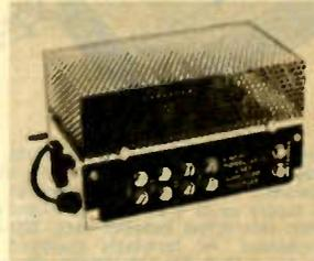
Model 65-1, boosts signal strength 8db low band-FM-and high band at each of 4 outputs feeding 4 VHF-TV or FM sets. With low loss splitters can feed 16 or more sets, depending on signal level and line length losses. Easily mounted with hardware provided. Features two 6HA5 low noise tubes, 300-ohm input and outputs with stripless terminals. 110v, 60 cps. 6 1/4x3 3/4x3 3/4".
