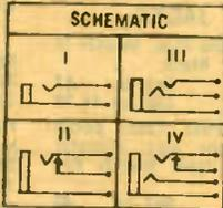
"LITTLE PLUGS" PHONE PLUGS—Compact quality plugs. Fits standard 1/4" phone jacks except \* with .206 diam. sleeve and † with short sleeve for Revere recorders. In plastic handle or with brass nickel plated shells for shielding. Solder terminal has built-in cable clamp. Handle 1 1/8" long, 1/2" diam. Av. shpg. wt., 4 oz.
