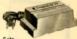
Model BC-83 boosts signal on all channels 2-83 plus FM from an 82 channel antenna. 300 ohm transistorized booster coupler designed to connect 2 sets using existing downlead. Average gain of 5.25 db to each output amplifies weak signals for snow-free reception. Silicon transistors for stability. 300-ohm input and outputs. No-strip terminals. Polystyrene case. 117 VAC.
