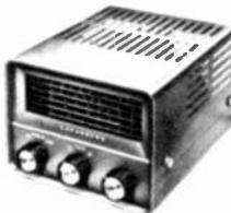
Employs a high "O" series tuned Clapp oscillator, remarkable for its low drift. A VR tube eliminates frequency shift due to variations in line voltage. High output of 10-20 volts is sufficient to drive any modern transmitter. Large easy-to-read illuminated slide rule dial with smooth tuning drive. Dual output impedance. Low heat silicon diode power supply prevents drain on transmitter power supply. Size: 6¼Wx5¼Hx7¼"D. For 117 volts 50/60 cps AC. Imported. Shpg. wt., 7½ lbs.
