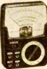
40  $\mu$ A, D'Arsonval meter movement permits a high input resistance on all ranges. Features a Mirror Scale. Rugged high impact plastic case. Ranges (DC Volts): 0-3, 30, 60, 300, 600, 3,000V; AC Volts: 0-6, 60, 120, 1200V. DC Current: 0-60  $\mu$ A, 0-12, 0-300 ma. Resistance: 0-60k, 0-6 megohms. Decibels: -20 to +63 db. Audio output jack. With test leads and 1 1/2 V battery. Size: 3 1/4 x 4 1/2 x 1 1/2". Imported. Shpg. wt., 1 lb.
