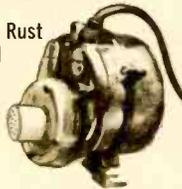
It's the all-new Deltron aluminum pump for underwater use. Guaranteed not to corrode or rust; hermetically sealed motor. Circulates and dispenses water and mild acid solutions, for use in fountains, beverage dispensers, aquariums, photo developing, air conditioning, etc. Gallons per hour delivery: 240 @ 1 ft.; 180 @ 3 ft.; 125 @ 5 ft., shut off @ 12 ft. Outlet ¾"; inlet ½" pipe O.D.; height 4½"; depth 4¼". 6 ft. safety cord. 115V AC, 60 cps, AC. 49 watts load; .67 amps load. Shpg. wt., ¾ lbs.
