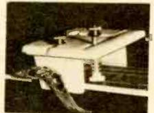
Provides that necessary "third Hand" for simple, accurate and rapid chain tuning.
