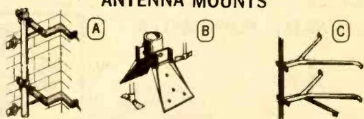
(A) CHIMNEY MOUNT An ideal chimney mount for life-long satisfactory service under the most severe conditions. "Z" type heavy gauge aluminum brackets. Complete mounting kit of two 12" stainless steel 3/4" straps and stainless steel seals. Rugged, corrosion resistant mount accommodates masts up to 1 1/2" O.D. Perfect for TV and FM antenna systems. Shpg. wt., 2 lbs. Net 2.95 18 P 6306
