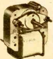
Rugged, GI open frame shaded-pole motor for continuous operation such as blowers, pumps, fans, animation, gear trains and many other hobbyist applications. 3500 RPM CCW rotation. Has oil-less type bearings. Shaft 3/16" dia. x 1 1/4" long. Body 2 3/4" wide x 3" high x 2" deep. Shpg. wt., 2 lbs.
