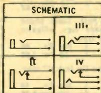
"LITTEL-PLUGS" PHONE PLUGS—Compact quality plugs. Fits standard ¼" phone jacks except \* with .206 diam. sleeve and † with short sleeve for Revere recorders. In plastic handle or with brass nickel plated shells for shielding. Solder terminal has built-in cable clamp. Handle 1½" long, ½" diam. Av. shpg. wt., 4 oz.
