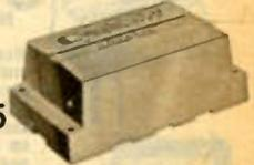
Model BC-03 boosts signal on all channels 2-83 plus FM from an 82 channel antenna. 300 ohm transistorized booster coupler designed to connect 2 sets using existing downlead. Average gain of 5.25 db to each output amplifies weak signals for snow-free reception. Silicon transistors for stability. 300-ohm input and outputs. No-strip terminals. Polystyrene case. 117 VAC.
