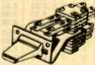
4PDT Audio Lever Switch: Has 2 dual sets of single pole, double throw contacts. One set is momentary contact-spring return, (press-to-talk). In the reverse position of the lever (dictate), the second set of contacts remain in the positive position until released. Panel mounting, mtg. centers 1" apart. Size 2 1/4" long behind panel. 1 3/8" W x 1"H. Imported. Shpg. wt., 3 oz.
