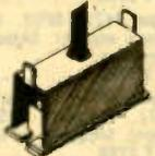
Exact replacement circuit breakers for television and industrial applications. Button must be pressed to reset. Tripping mechanism is temperature compensating for constant protection. Normal tripping time is 10 seconds or less. All values above 3.1 amps have special heavy-duty contacts to withstand heavy surge currents. Twist tab mounting lugs. Adapter for bushing mount listed below.
