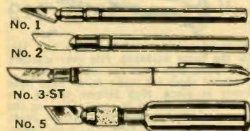
X-ACTO interchangeable-blade, precision knives for: carving, cutting, hollowing, scribbing, stripping, trimming, etc. Heavy-duty handles for rugged service. Avg. shpg. wt., 2 oz.
