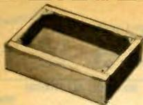
Chassis are of one piece construction with gussets spot-welded to the bottom flanges for additional strength. Made of No. 18 gauge (.040) aluminum except † are No. 14 gauge (.064) in natural aluminum finish.
