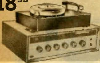
4-speed (16, 33 $\frac{1}{2}$ , 45, and 78 RPM) phono-graph turntable is designed to fit on top of the amplifier and is easily mounted with two screws. Fits snugly over amplifier. Takes records up to 12". High quality ceramic pickup—turnover type with dual synthetic sapphire stylus. Power requirements: 15 watts. 117 volts 60 Hz AC. Durable finish matches amplifier. Size: 12 $\frac{1}{2}$ "x8 $\frac{1}{2}$ "x4". Shpg. wt., 8 lbs.
