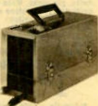
Hundreds of uses: Operates TV's, power tools, barbecue motors, lights, hedge clippers, or appliances using 117V., 60 Hz AC. Has self-contained 25 amp, rechargeable wet storage battery. Frequency stable within ½ cycle with load changes. Plugs into AC outlet, or, car cigarette lighter to recharge battery. Has automatic overcharge protection. Meter shows charge rate and hours of anticipated output. Size: 12x5½x8". Shpg. wt., 36 lbs.
