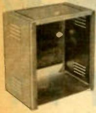
16 Gauge steel cabinet racks. Front vertical corners are rounded and the top and bottom are trimmed with red striped chrome finished moulding. Recessed piano-type hinged door in top. Units marked \* also have hinged rear door. Louvered sides and rear opening provide ventilation. Panel mounting holes tapped for 10-32 machine screws. Gussets welded at bottom of rear on types 170-350 for additional strength. All are 21 3/4" wide, 15 1/4" deep. Finished in gray hammertone. o/a = overall.
