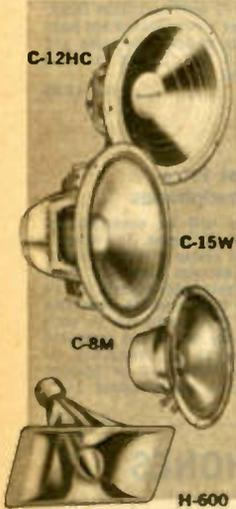
**MODEL C-12HC 12" HIGH COMPLIANCE WOOFER.** Impedance, 4-20 ohms. Freq. response 20-30,000 Hz. Rated at 50 watts. Cone resonance 20 Hz. 6 7/8" deep. Shpg. wt., 9 lbs.
