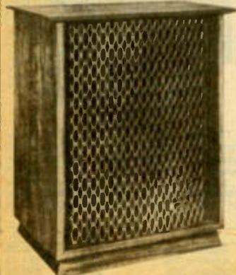
Magnificently styled, two-way speaker system in a hand-rubbed, oiled walnut finished floor model cabinet with 16th century Spanish style fretwork wood grill. Features a 414A, powerful 12" low frequency speaker; 3000H high frequency driver; cast zinc multicellular horn; and N-3000E two section crossover network. Frequency Response: 40-22,000 Hz. Crossover: 3000 Hz. Power Rating: 20 watts. Impedance: 8 ohms. 26H x 19W x 14"D. Shpg. wt., 60 lbs. 11.50 Monthly
