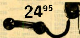
Modernize your present fixed or mobile CB station with these telephone style handsets. Attaches to dashboard, side of unit or wall of fixed station. Switch in the cradle automatically disconnects the speaker when the handset is lifted. The microphone is activated by means of a push-bar, push-to-talk switch. Ideal for use in heavy traffic, loud background noise area, at home or in the office for privacy. Shpg. wt., 2 lbs.
