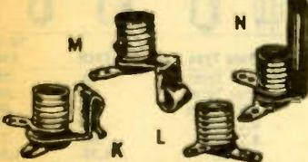
Cadmium plated brackets with tinned brass lugs. Bayonet type with coil spring construction for positive contact. For miniature screw, bayonet, and candelabra base. Threaded jewel assemblies may be used with these sockets to provide panel indicators, and are listed above. Av. shpg. wt., 2 oz.
