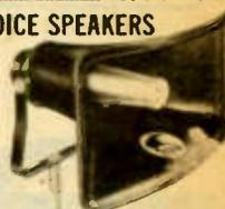
Model CJ-40. Voice speaker. Attractive charcoal gray, molded fiberglass. Minimizes feedback, boom, and annoying harmonics to create performances that can be heard. 40 watts peak music power. Can be mounted on any mike stand (see p. 181) or with model SS-4 stand below. Quick connect/disconnect receptacle takes standard phone plug. Response: 150-14,000 Hz. Impedance 8 ohms. 6H x 14W x 12¾" D. Shpg. wt., 9 lbs.
