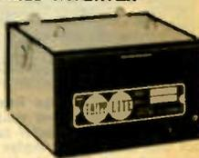
Model PV-100. Designed to give instant AC power where fast emergency service is needed. Lightweight, low-cost inverter converts 12 volts DC to 115V., 60 cycles AC; delivers 100 watts continuously. Specifically engineered to power televisions, and tape recorders in cars, boats, planes, or mobile homes. Incorporates 2-power switching transistors. Complete with cigarette lighter plug, and standard AC outlet. Size: 4 3/4 x 4 3/4 x 3".
