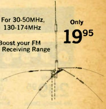
An exceptionally efficient ground plane antenna for operation between 30 to 50MHz and 130 to 174 MHz. Comprised of 4 easily assembled drooping elements tuned to 30 MHz and a vertical radiator with a matching transformer and a low and high band collinear collector. Ideal for use with Lafayette FM communications receivers. Constructed of heavy-duty aluminum alloy rods and stainless steel tip section. Antenna comes complete with mounting bracket for 1" pipe or 1 1/4" tubing. Shpg. wt., 6 lbs.
