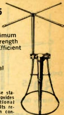
"Astro-Plane" base station antenna provides full omni-directional communications. Its revolutionary design concentrates signal power on top for maximum, efficient operation. Heavy duty aluminum construction with corrosion resistant fittings, including solderless coax connector, assure a long, trouble free life. Double bracing withstands 120 mph winds. Impedance: 50 ohms; SWR: less than 1.4/1; power gain: 4 db; length: 12'. Can be mounted on a single mast up to 1 1/2". Shpg. wt., 4 lbs.
