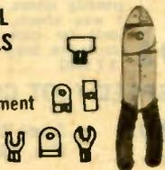
A complete crimp tool kit for home, shop. Solderless terminal crimp tool cuts any size wire up to 10 gauge, strips wire easily with clearly marked gauges. Crimps terminals quickly with precision tooled crimping dies. Easy to use with comfortable insulated handles. Complete with plastic box of assorted solderless terminals and connectors. Imported. 13 T 7000 Shpg. wt., 1 lb. Net 2.19
