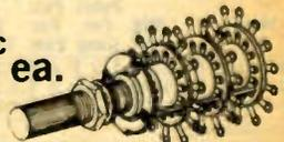
Non-shorting type with 3 circuits per gang or section. Rated current capacity is 50 ma at 100 VAC. Insulation resistance 100 megohms at 500 VDC. Contact resistance without load is 1/100 ohm at 6 VDC. Perfect for transistor applications. Mounting depth is 1 1/2". Imported. Shpg. wt., 4 oz.
