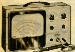
Deluxe peak-to-peak VTVM for all TV/FM/AM servicing. Features big 7½" meter in "can't burn out" circuit. Has zero center scale, 1% multiplier resistors and "Uni-probe" for all measurement functions. Ranges: p-p volts, 0-4-14-42-140-420-1400-4200 v; DC/RMS volts, 0-1.5-5-15-50-150-500-1500 v. Response, 30 Hz to 3 MHz. Resistance, 0.2 ohms to 1000 megohms in 7 non-skip ranges. Size: 8½x13x5". For 105-125 v. 50/60 Hz AC. Shpg. wt., 9 lbs.
