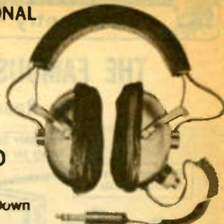
Rugged construction makes it both shatterproof and shockproof. Adjustable, spring steel headband and fluid filled ear cushions are designed to fit head contour, thus forming a more efficient seal for almost complete attenuation of ambient noise. High quality drivers mounted in acoustically designed enclosures provide smooth frequency response from 30 to 20,000 cps. Removable cushions can be cleaned with soap and water. With 10 ft. coiled cord and plug, 4 ohms impedance. Shpg. wt., 3 lbs.
