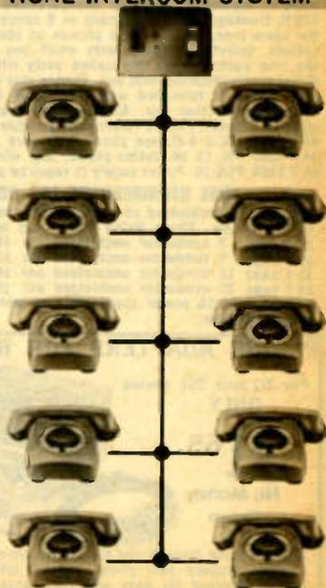
In the above 10-station system up to 5 private conversations can be held simultaneously—or any station may converse with any other station.
