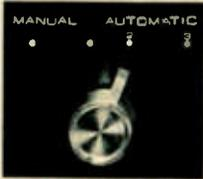
**1) MANUAL**—Same as any tape recorder, but permits manual reverse at any point by depressing a button. Sensing metallic foil is disregarded.
