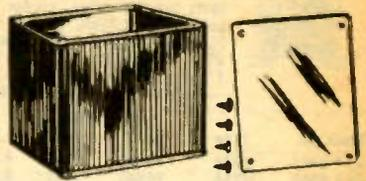
Made of aircraft alloy aluminum, drills and machines beautifully. Patented lock-joint corners tighten under stress. Six flat parts assemble easily with screwdriver; 2 flinned sides have .100" max. wall for use as heat sink; 2 plain sides have .040" wall. Strong and rigid, will withstand 2-tons. Easily mounted above or below chassis. Avg. Shpg. wt., 2 lbs.
