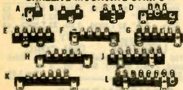
Cadmium plated steel lugs spaced 3/8" on centers. Bakelite strip is 3/8" wide x .062 in. thick. Ideal for supporting and joining electrical components. Type marked \* have grounding lugs in addition to the number of terminals indicated below. Mount with No. 6 screw. Avg. wt., 1/2 lb. 5 per pkg.
