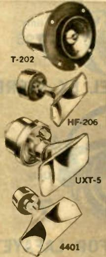
**MODEL T-202 SPHERICON SUPER TWEETER.** 3,000-40,000 Hz. (±2 db to 22,000 Hz). Domed phenolic diaphragm with spherical diffractor. Built-in network and brilliance control. 8 ohms, 30 watts. Shpg. wt., 3 lbs.
