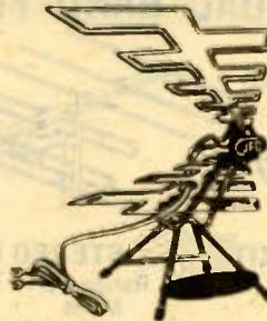
A log periodic UHF indoor antenna—with electronically tuned brass-plated trapezoid dipoles. Frequency-independent design pulls in extremely strong signal on all channels 14 to 83. Sharp unidirectional beamwidth removes snow, rejects ghosts and interference. Unusually low VSWR, 300-ohm twin lead. Tip resistant, rubber cushioned stand. Shpg. wt., 3 lbs.
