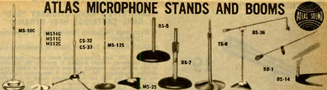
**Model MS-10C Full Grip Mike Stand.** Economical mike stand featuring "Full-Grip" clutch mechanism for fast quiet adjustments without slipping and wear. Functionally designed base assures maximum stability and includes self-leveling, shock-absorbing pads plus 3 "anti-tip" points. Full chrome plated tube assembly. Terminates in a 5/8"-27 thread. Base dia. 10", finished in gray shrivel. Height adj., 35 to 63". Shpg. wt., 10 lbs.
