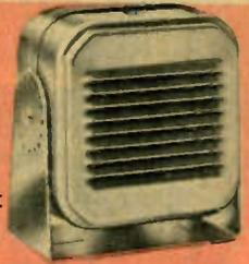
Model MS-3B. Compact, weatherproof, dustproof. Ideal for use in mobile communications, for intercom paging, and as an extension speaker. Can be immersed in water. Power rating 3-watts. Resp 100 to 10,000 Hz; 8 ohms imp. 4½ x 4½ x 2¾ with bracket. Wt., 2 lbs. 44 C 5201 Net 6.49
