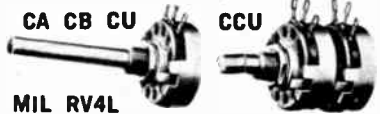
TYPE CU MIL RV4L Locking type with nut and slotted shaft. 1 1/2" dia. All have linear taper.
