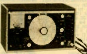
Features 100% silicon transistor circuitry, zener-regulated power supply, 6-individually shielded step attenuators, variable line output level control, and calibrated 200  $\mu$ A D'Arsonval meter. Range: 100 kHz to 54 MHz on fundamentals (5 ranges), and 54 to 216 MHz on harmonics. Outputs: modulated RF, unmodulated RF, external modulated RF, 400 Hz audio. For 110-120V., 60 Hz AC. Size: 12 3/4 x 7 1/2 x 8" D. Shpg. wt., 16 lbs. 38 F 17319WX No Money Down\* Net 159.95
