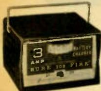
Full 3-amp battery charger for quick starts in all weather. Edge view colored meter shows actual battery condition. Reset circuit breaker gives automatic overload protection. Has 6 and 12 volt selector switch. Delivers tapering charge. Vented steel case; may be wall mounted. 6 ft. battery leads with 50 amp clips. Size: 6 x 4 $\frac{1}{2}$  x 5 $\frac{3}{4}$ ". For operation from 105-125 Volt, 60 Hz AC. UL Listed. 11 F 76049 Shpg. wt., 5 lbs. Net 10.95
