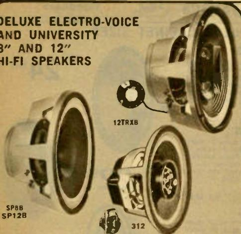
**ELECTRO-VOICE SP8B RAOX SUPER EIGHT**—8" speaker. Resonance 60 Hz. Power rating 20 watts. Response 35-15,000 Hz. 16 ohms impedance. Sens. Rtg. 47 db. Crossover 4500 Hz. 1 lb. 6 oz. ceramic magnet. 8 $\frac{3}{4}$ " diam., 7" baffle opening. 4 $\frac{3}{4}$ " depth behind panel. 21 F 30599 W Shpg. wt., 9 $\frac{1}{2}$  lbs. Net 32.50
