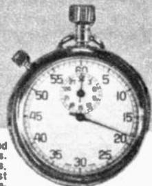
Second hand registers 1/5 of a second and completes turn in 60 seconds. Small hand indicates up to 30 minutes. Side slide starts and stops hands. Fast resetting, dependable 7-jewel movement. Imported. Shpg. wt., 6 oz.
