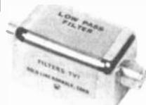
Avoid TV interference. Reduce TVI coming from your rig and interfering with TV sets by inserting an LP filter in your line. Rated at 100 watts input. Attenuation starts at 39 MHz, is 20 db down @ 40 MHz, 26 db @ 45 MHz and above. Impedance: 50 ohms. Insertion loss: 1/2 db @ 27 MHz. Shpg. wt., 3/4 lb.
