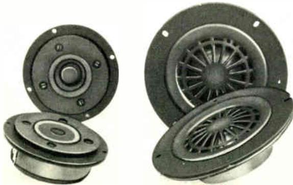
**Matched Pair of High-Power Dome Hi-Fi Tweeters.** Here's high powered 3½" tweeters with dome-shaped diaphragms, perfect for adding on to existing speaker systems. Negligible transient distortion with low cone mass. Magnet: 9 oz. Crossover: 4000 Hz. Handles 40 watts. 1500–20,000 Hz. Holland. Mail wt., 3.0 lbs.
